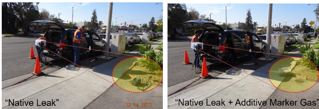
Figure 4 – Performing methane emission quantification at a targeted address, 1) measuring the native methane emission, and, 2) measuring the native methane emission with additive marker gas included.
