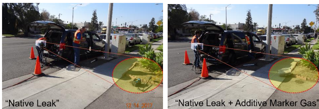
Figure 4 – Performing methane emission quantification at a targeted address, 1) measuring the native methane emission, and, 2) measuring the native methane emission with additive marker gas included.
