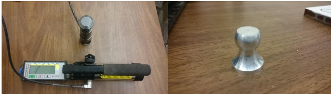
Figure 7 Manual adhesion tester and dolly
