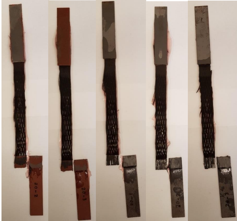
Figure 21 Specimens after failure (from left to right): Coated-20-2, Coated-20-3, Uncoated-20-1, Uncoated-20-2, Uncoated-20-3.
