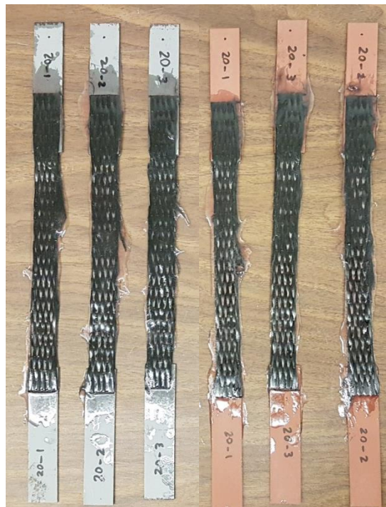
Figure 20 Lap-Shear specimens prepared: uncoated (left) and coated (right).
