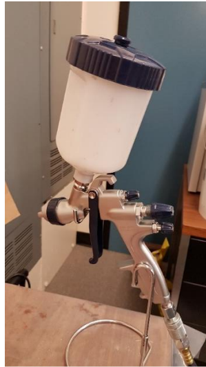
Figure 13 HVLP spray gun for coating spray
