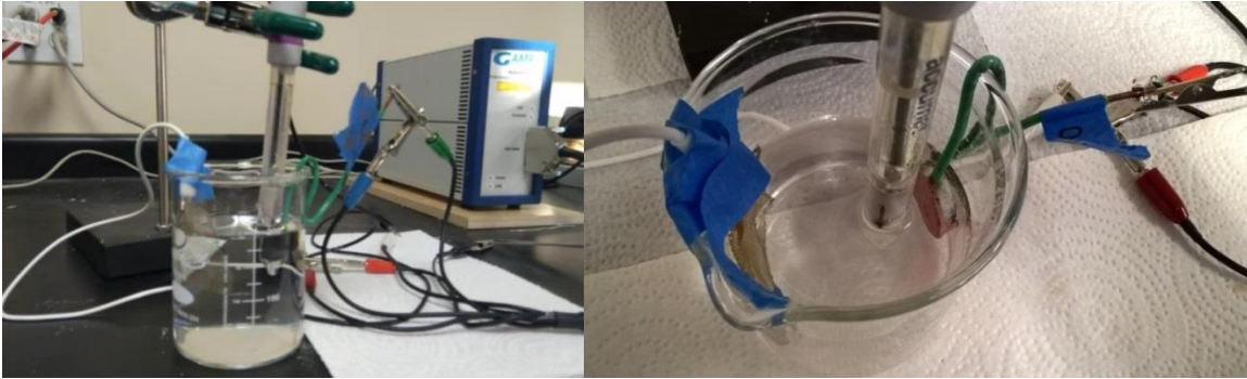
Figure 2 EIS testing with coated sample
