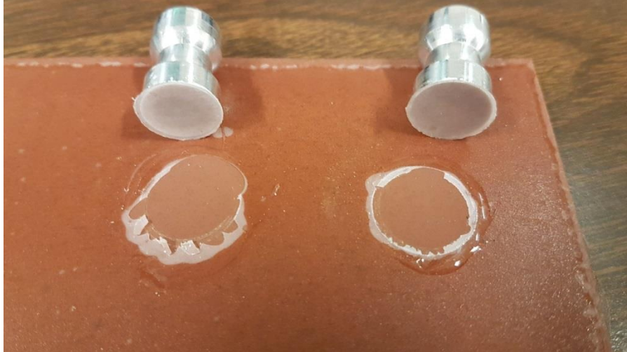
Figure 22 Pull off strength performed on coated steel specimen topped with DowAksa CarbonBond 300H Saturant Resin
