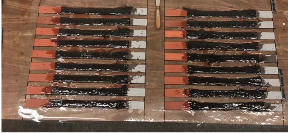
Figure 23 Samples prepared for lap shear test
