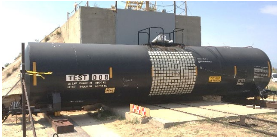
Figure 1. Pre-test Photo of DOT-105 Tank Car
