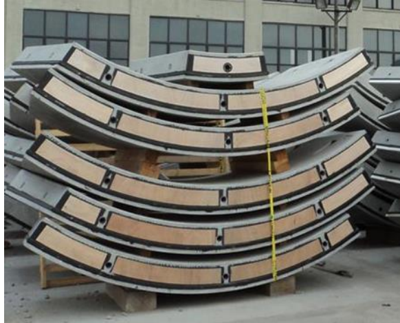
Figure 5-4: Example of load distribution plates on the circumferential face of segments. Photo: FHWA.
