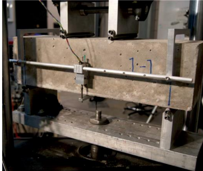
Figure 6-1: Deflection controlled four-point-beam test per ASTM C1399 (ACI 544.8R). Photo courtesy ACI.
