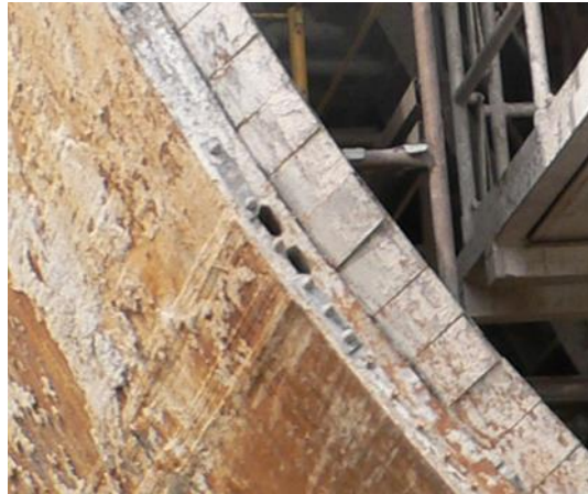
Figure 5-5: Backfill grout dual port outlet embedded in the shield of a large diameter TBM. Photo: FHWA.
