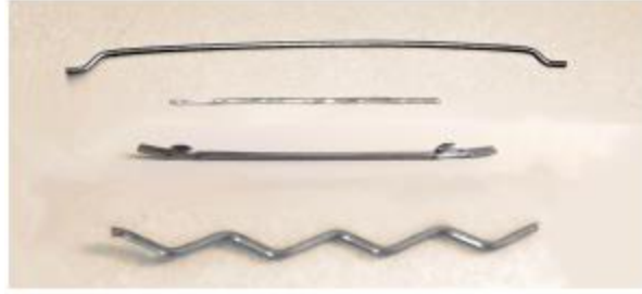
Figure 4-7: Types of steel fibers with anchors. Photo: FHWA.
