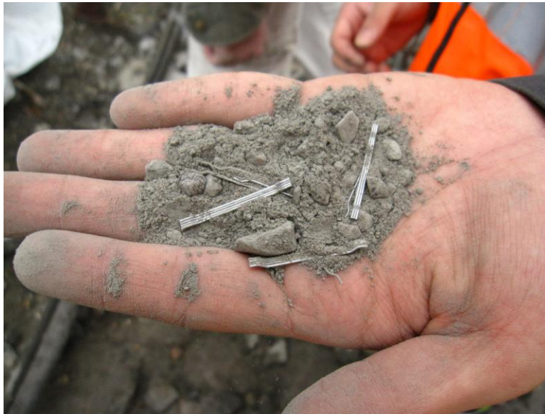
Figure 4-6: Dry concrete mix with steel fiber reinforcement. Photo: FHWA.
