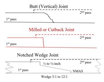
Figure 3. Longitudinal Joint Types.
