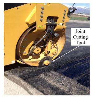
Image: Adam Hand Figure 9. Joint Cutting Tool on Compactor.
