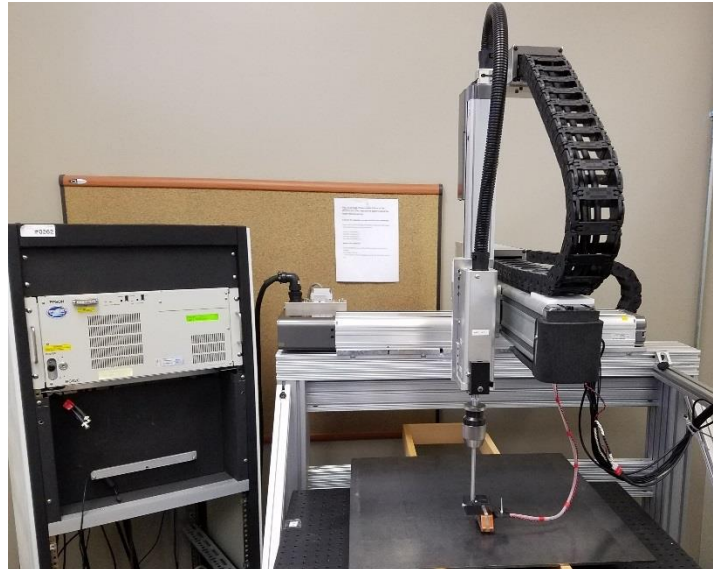
FIGURE 5. EPSON 3-STAGE SCANNING ROBOT WITH FLAT PLATE MREC.
