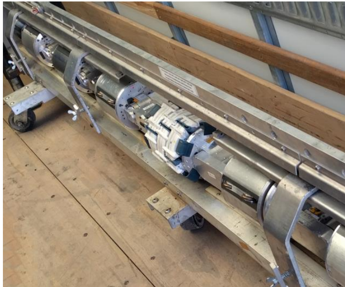
FIGURE 35: AMR EC SENSOR ABOARD 8IN EXPLORER
