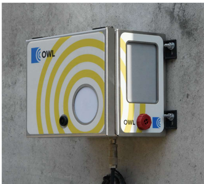
Figure 3 - Operator Warning Light (OWL)
