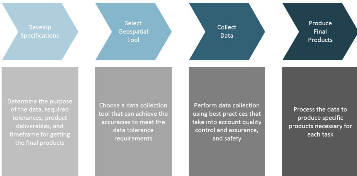
Figure 3-2. Flowchart. General guidance for effective use of geospatial tools in highway construction projects.
