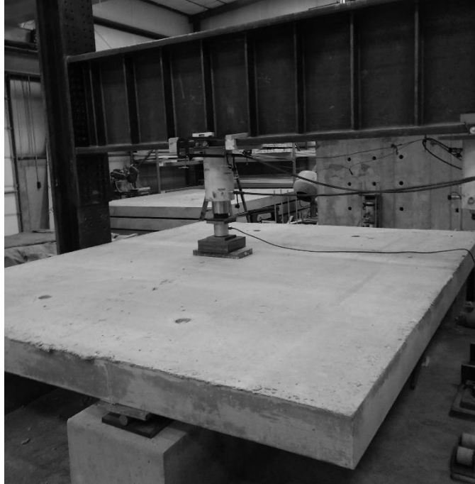
Figure 4.3.13 GFRP punching shear static test setup
