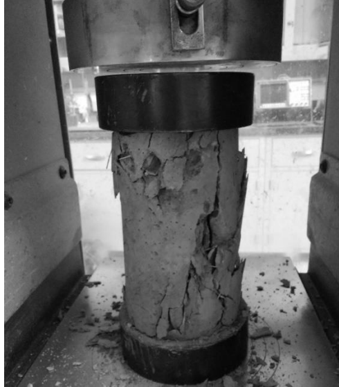
Figure 3.2.9 Compression test of an FRC cylinder
