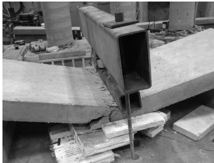
Figure 7.4.11 HRC failure after 2 million cycles
