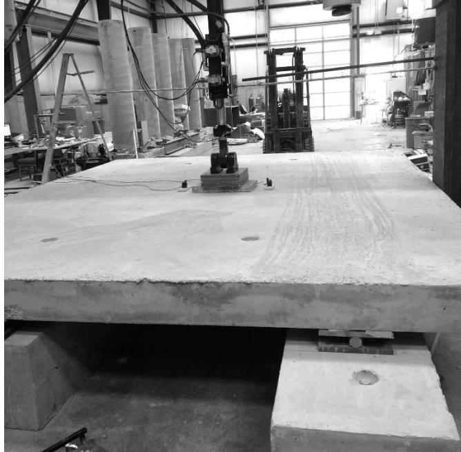
Figure 4.3.16 Fatigue test setup 2
