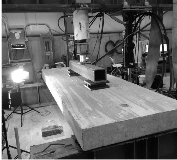
Figure 3.3.12 Static test setup (steel-reinforced deck)
