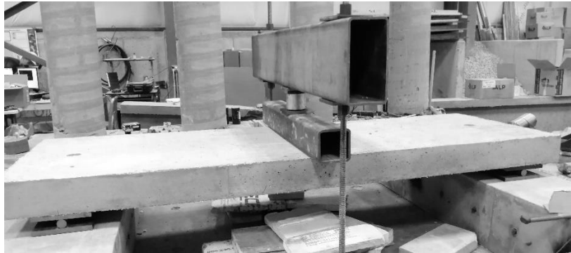
Figure 3.3.18 Static test after fatigue loading
