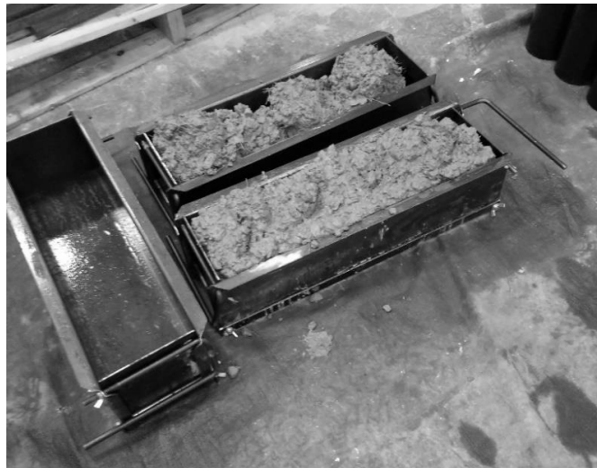
Figure 3.2.3 Filling up the mini beam molds
