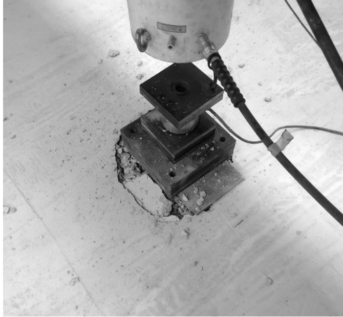
Figure 8.4.7 Top of HRC post-fatigue punching shear deck
