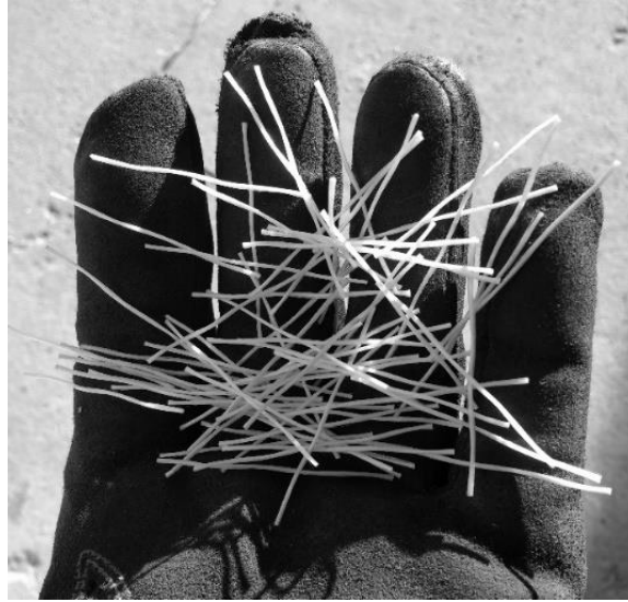
Figure 3.2.7 Macrofibers used in this experiment
