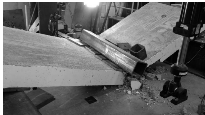
Figure 7.4.16 GFRP deck at failure
