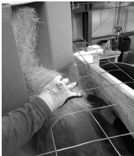
Figure 3.2.8 Adding fibers through a grate to prevent clumping
