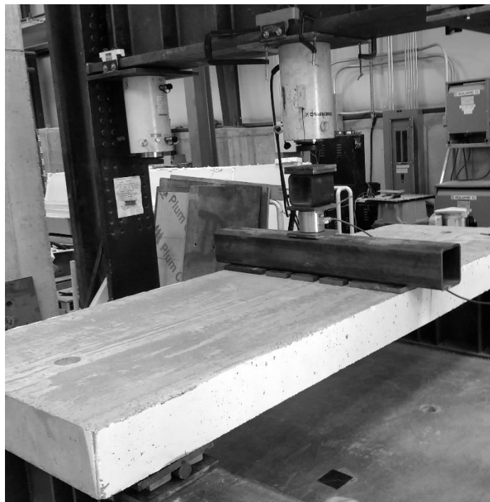
Figure 3.3.13 Static test with centerline loading (GFRP deck)
