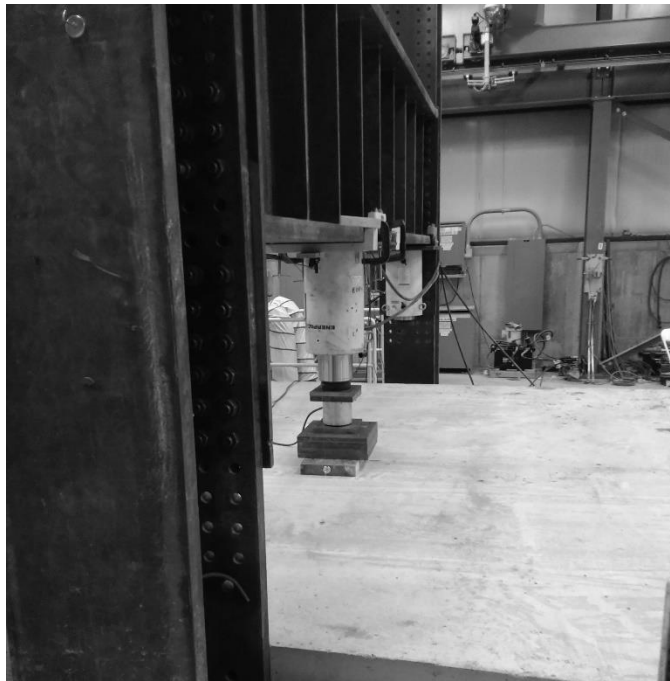
Figure 4.3.14 HRC punching shear static test setup
