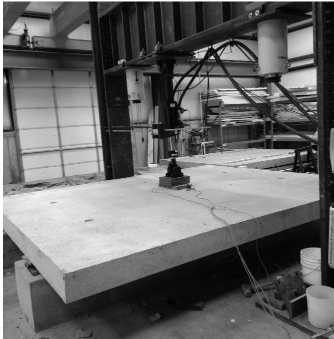
Figure 4.3.17 Fatigue test setup 3
