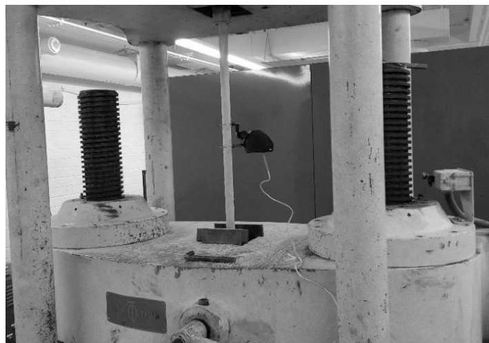
Figure 3.2.4 GFRP tensile test setup
