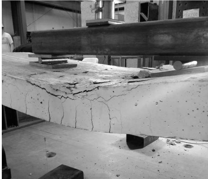
Figure 7.4.15 Steel deck at failure
