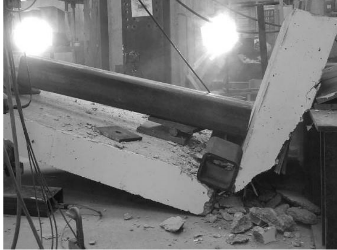
Figure 7.4.10 Shear failure on first GFRP specimen
