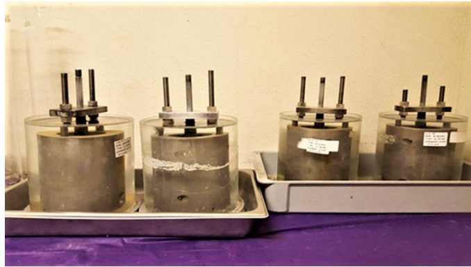
Figure 6.2 The saturation of Na-MMT clay samples using four controlled uniaxial swelling (CUS) devices
