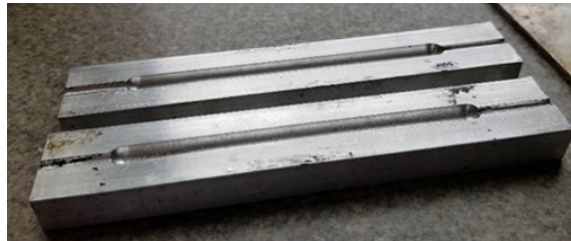
Figure 4.4: Mold for compression molding polyethylene tube specimens.
