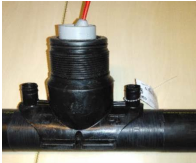
Figure 15 The Spatial Requirements and Fit Tolerance was Verified Prior to Live-gas Testing
