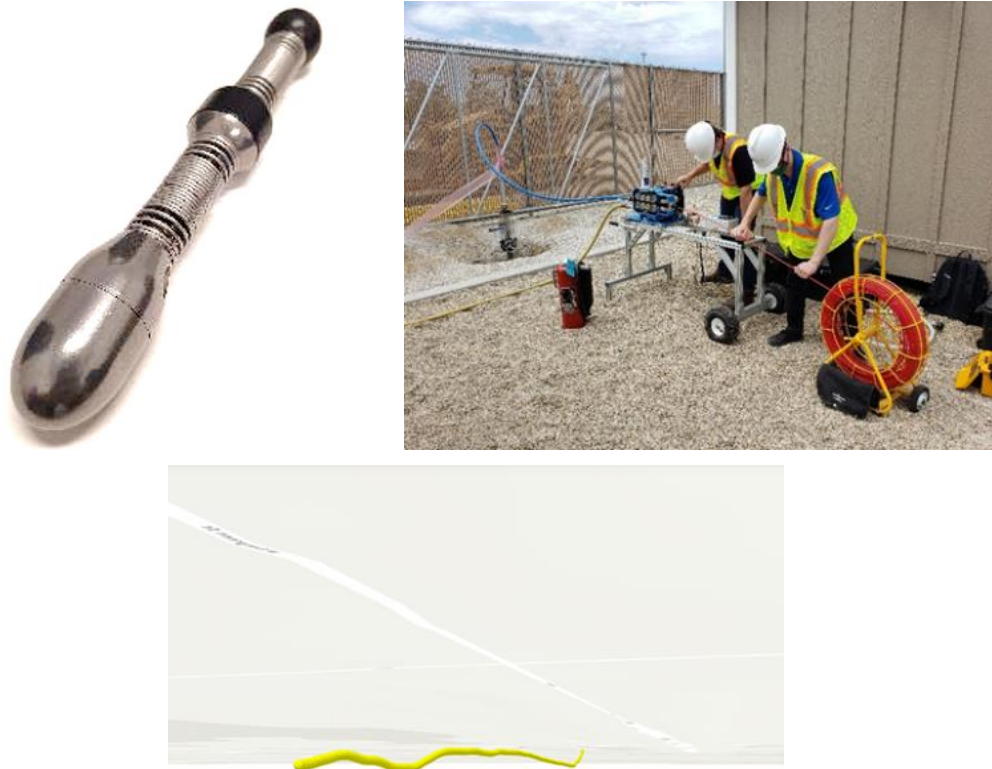
Figure ES 1: The Mapping Probe, Integrated System of Propulsion, and 3D Data Output
