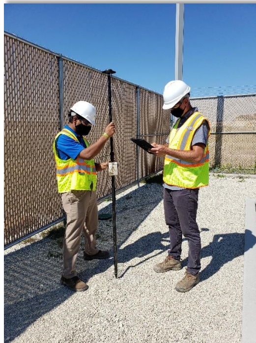
Figure 48: A high accuracy GNSS Receiver attached to a survey pole and accompanying tablet
