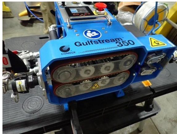
Figure 31 Pneumatic Duct Rod Pusher Mechanism
