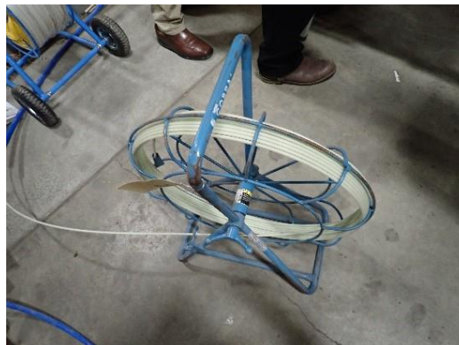
Figure 32 Image of Duct Rod Spool used for Propulsion
