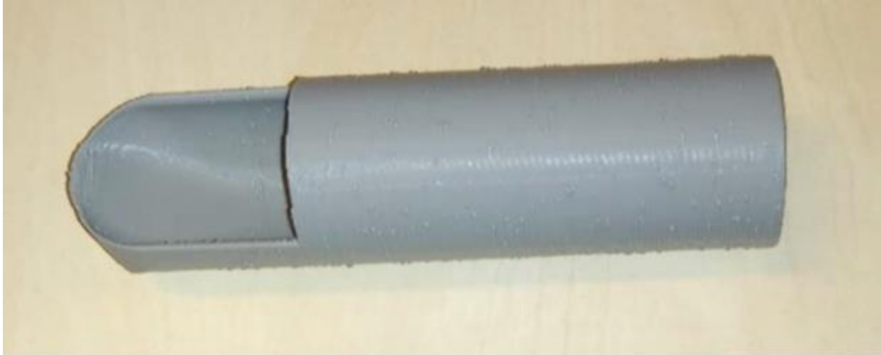
Figure 14 Initial Design Concept of Insertion Shoe for Live-gas Entry
