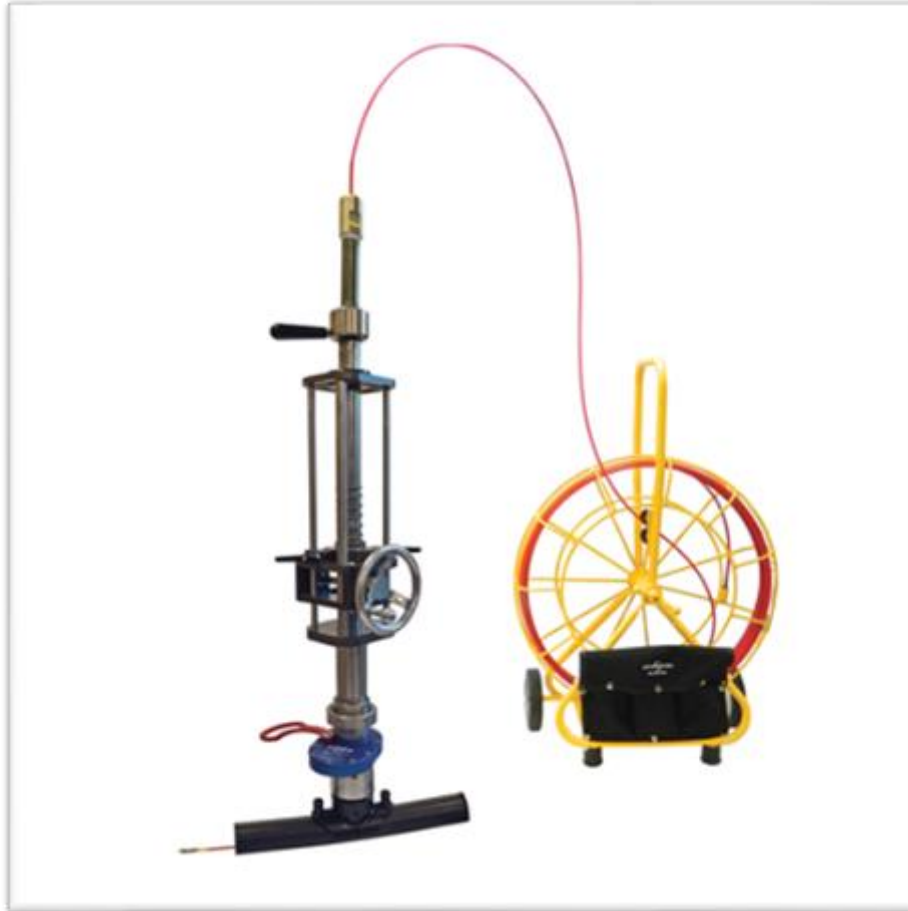
Figure 25 Jameson Live-Gas Launch Tool and Pipeline Access Fittings
