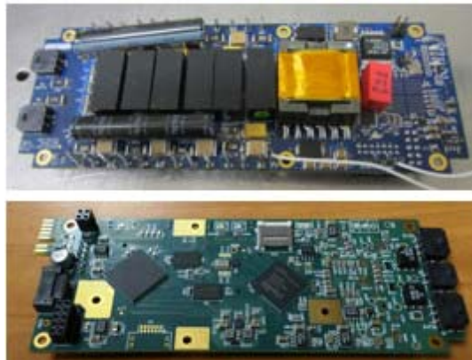
Figure 16. Pulser PCB (A) and Receiver PCB (B)
