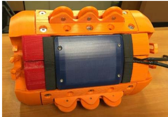
Figure 12. Fit Check of the Sensor Carrier Subassembly with the 3D Printed Sensor Module Housing
