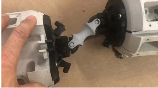
Figure 40. 3D Printed prototype for Link between Modules
