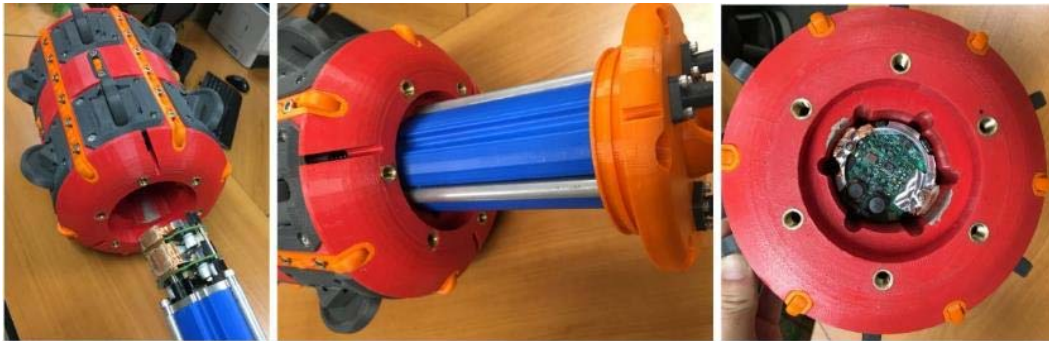
Figure 20. Power Supply Fit Check on a Battery Module Housing Mockup
