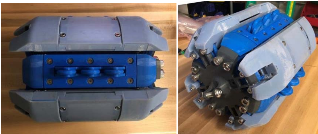
Figure 10. 3D printed EMAT Sensor Module. Top View (left) and Isometric View (right).
