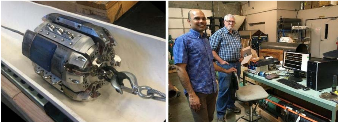
Figure 27. EMAT/CRACK Sensor Module (left), and Test Setup (right)
