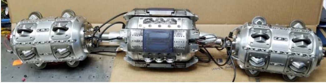
Figure 22. Assembled and Connected EMAT/CRACK Tool
