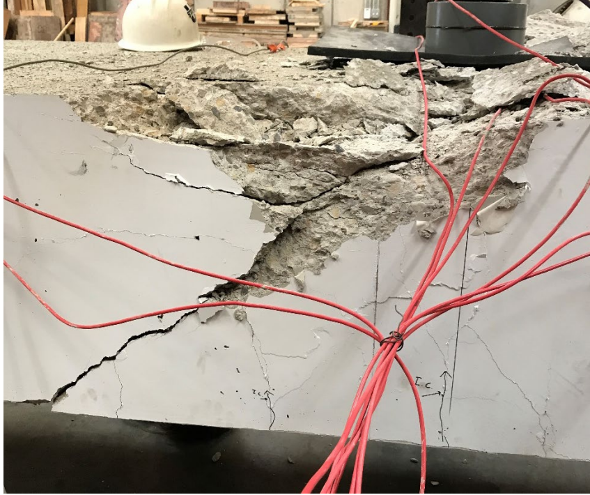
Figure 6.2 Midspan Test Failure Mode
