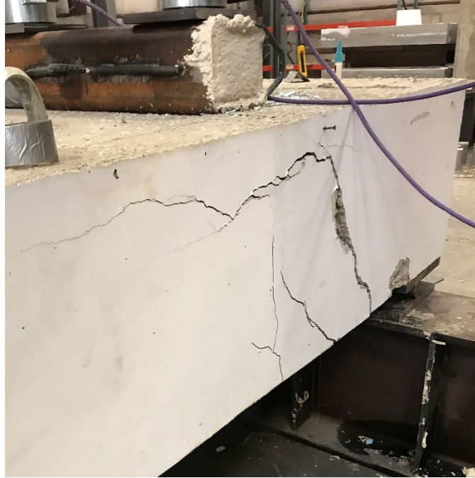
Figure 7.2 Failure of 1.25d Testing North Face
