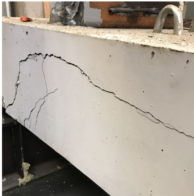
Figure 7.3 Failure of 1.25d Testing South Face
