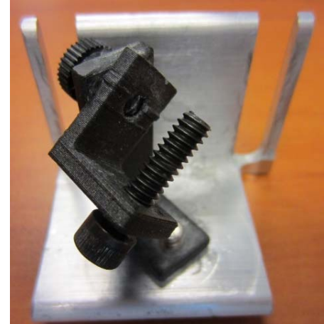
Figure 4: In-house designed and manufactured 3-axis goniometer.
