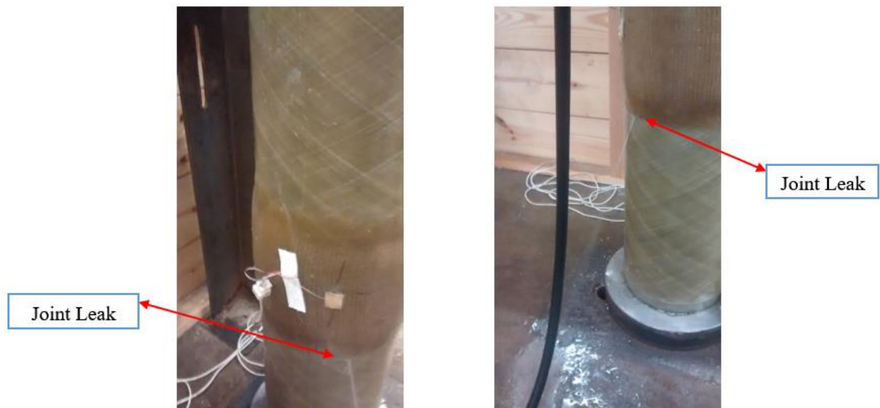
Figure 3-2: Butt joint failure
