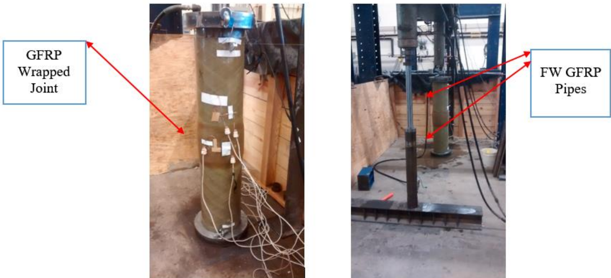
Figure 3-1: GFRP butt joint pressure testing
