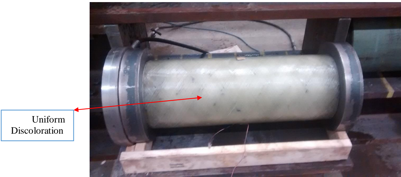
Figure 2-17: 3/4 wall specimen 1 discoloration
