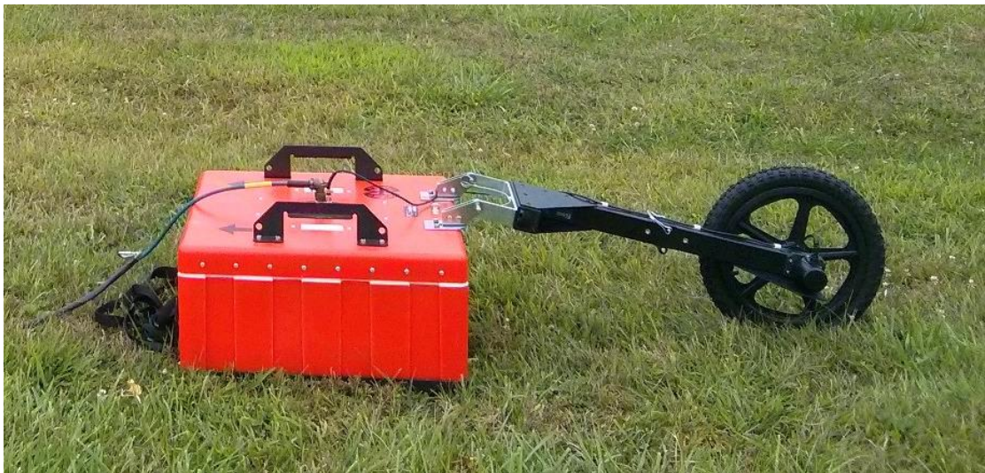
Figure 5-2: 200 MHz GPR antenna with survey wheel
