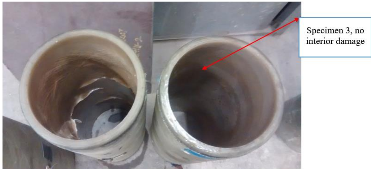
Figure 2-20: Interior damage of specimen 1 and 3
