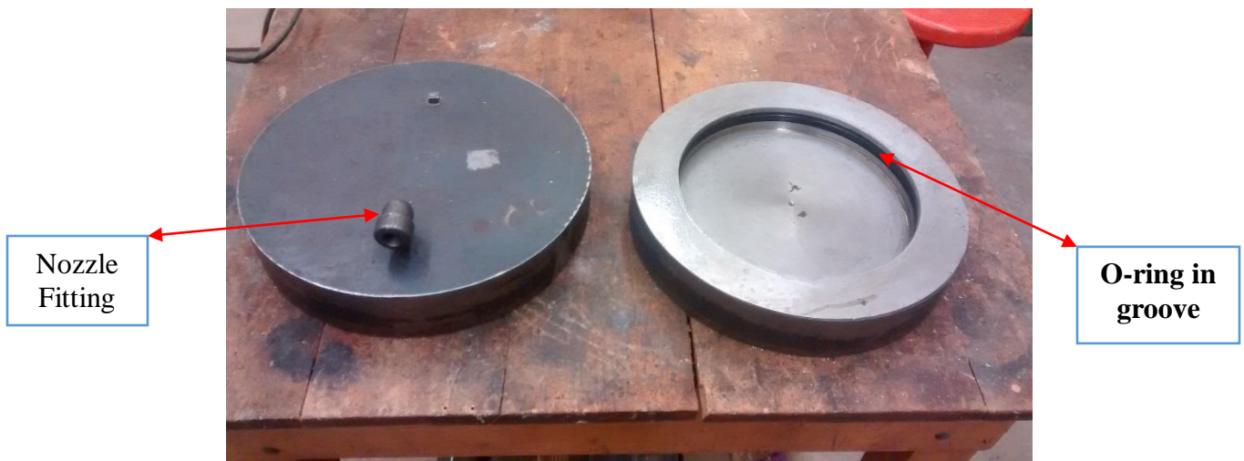
Figure 2-3: Steel endcaps for 10 inch od pipe
