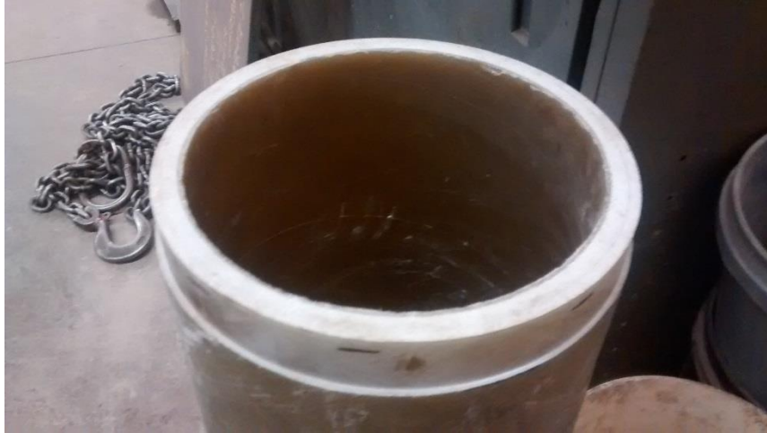
Figure 2-4: Machined pipe ends
