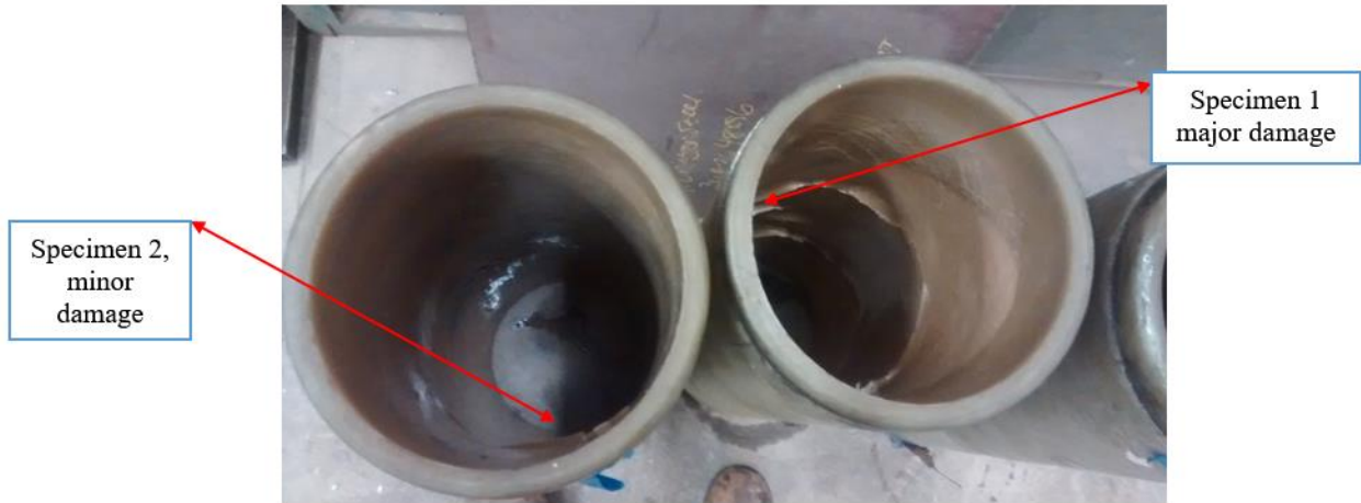
Figure 2-19: Interior Damage of Specimen 1 and 2
