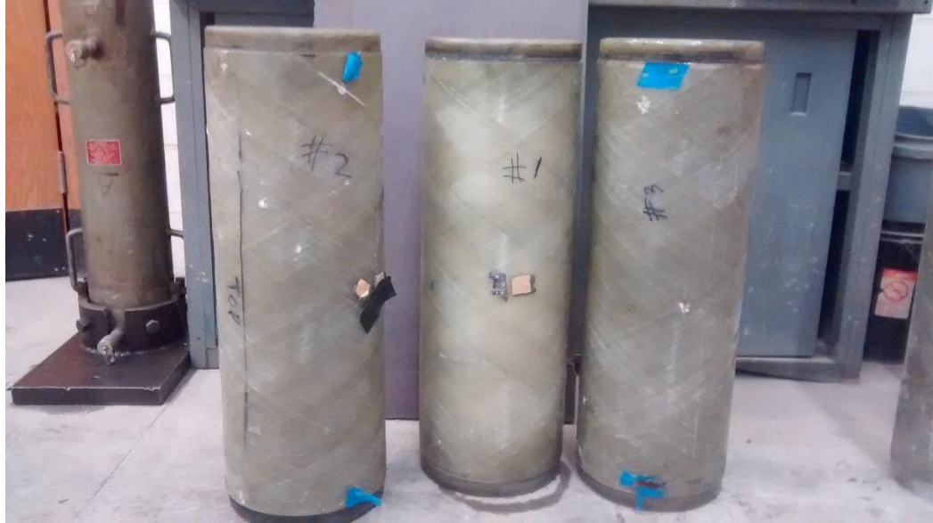
Figure 2-18: Exterior damage of thick walled pipes
