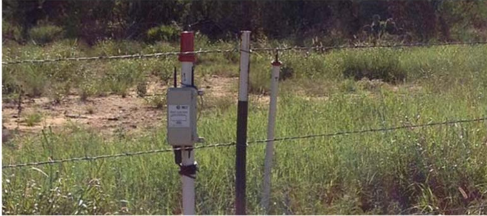
Figure 6 – Example of RPMA End Point in the Field
