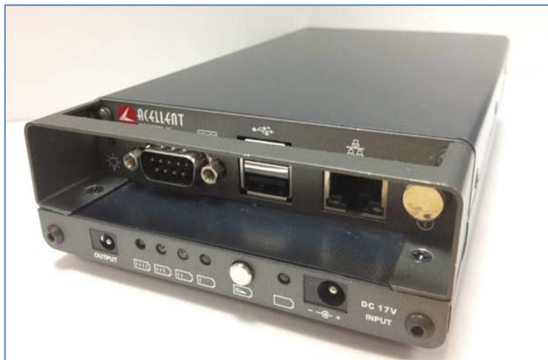
Figure 12. Accellent Technologies Vibration Signal Processor
