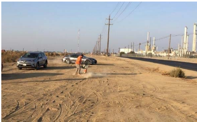
Figure 53. Vibration Test with Compactor
