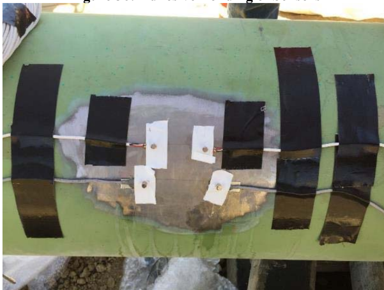
Figure 36: Adhesive Bonding of Sensors
