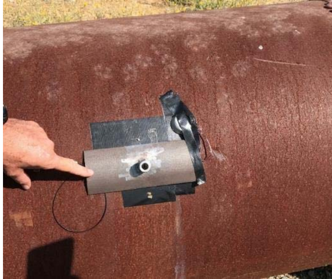
Figure 19. Field Shielding Developed for Pipe Sensors
