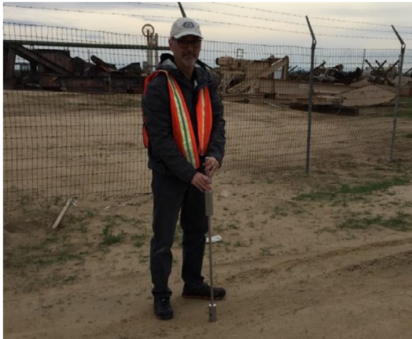
Figure 82. DCP to Generate Impact Signal
