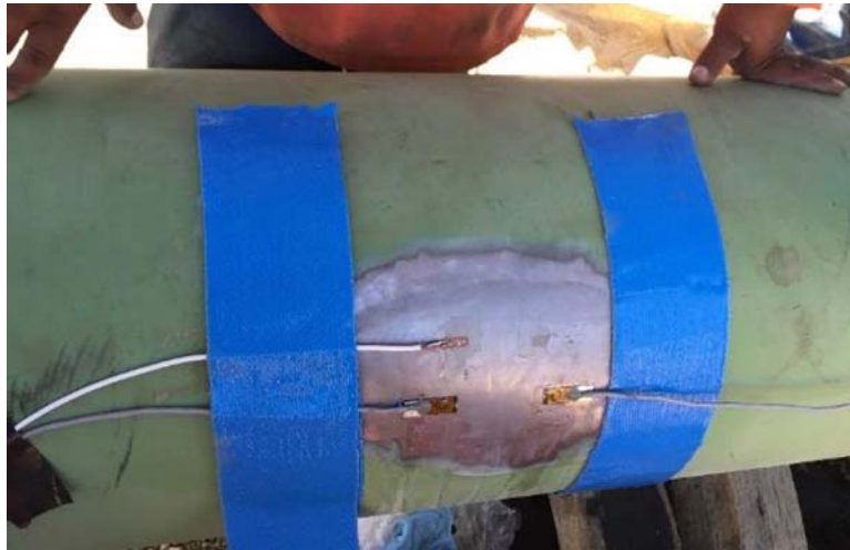
Figure 29. Form Protective Patch over Sensor Area
