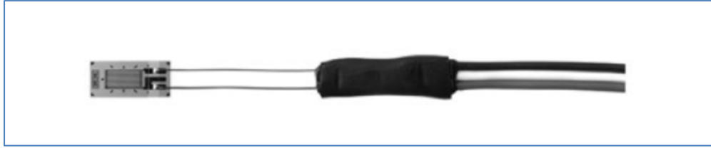
Figure 17. Adhesive Bonded Strain Gauge with Cable
