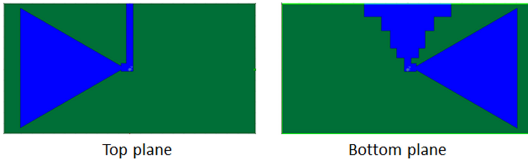
Fig. 2.28. Bow-tie antenna of 1) Top plane and 2) Bottom plane (Board size 60cm*116cm).
