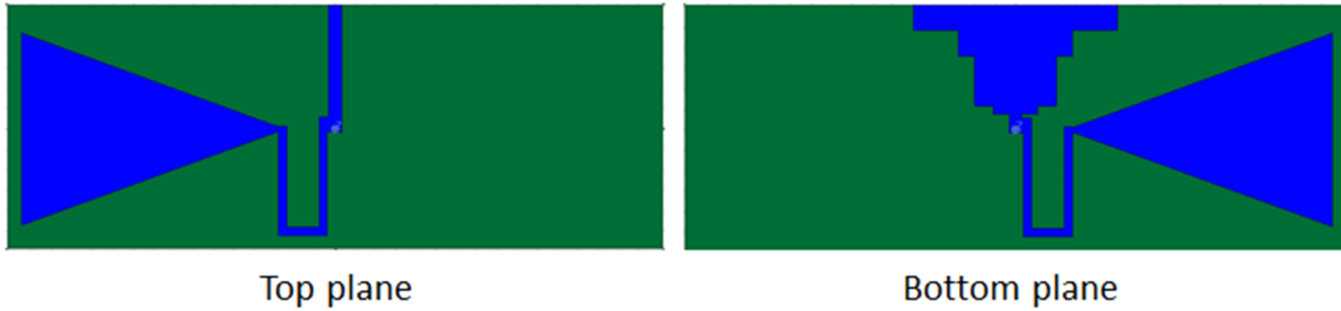
Fig. 2.30. Meandered bow-tie antenna of 1) Top plane and 2) Bottom plane (Board size 60cm*162cm).
