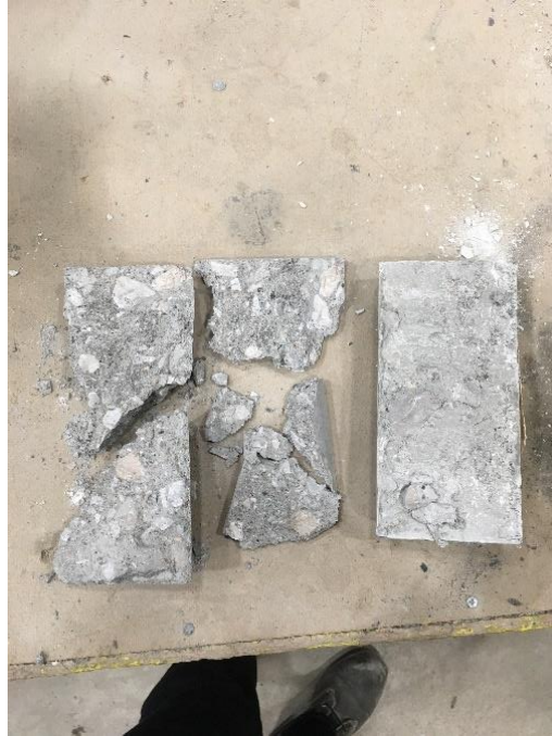
Figure 5.27. Cylinder 3 split cylinder failure
