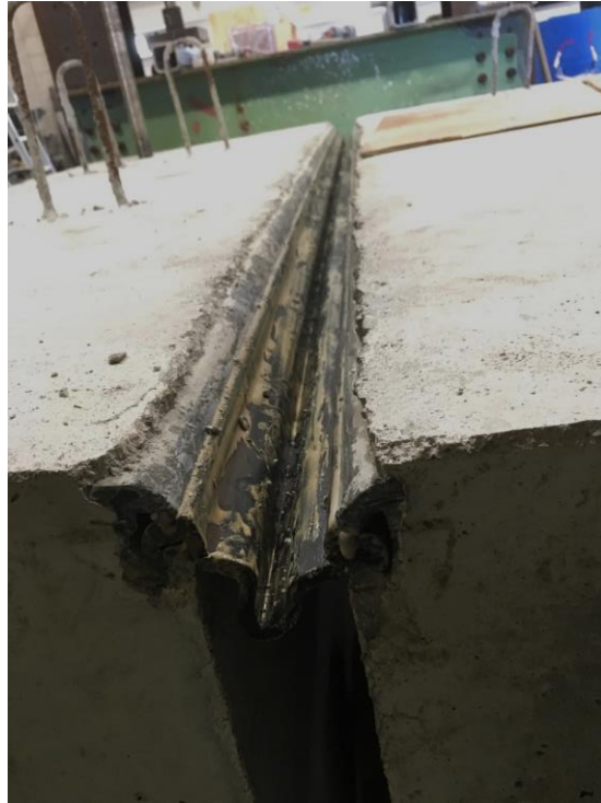
Figure 5.1. D.S. Brown A2R-400 strip seal
