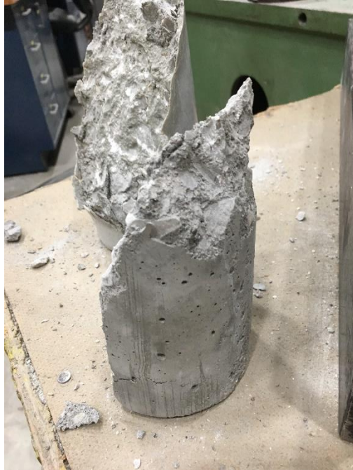
Figure 5.21. Cylinder 2 slant shear failure
