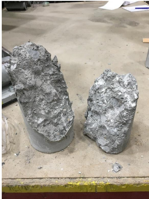
Figure 5.22. Cylinder 3 slant shear failure
