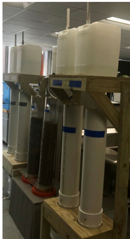
Figure 6.6: Duplicate Experimental Setup with 6-inch Diameter PVC Tubes
