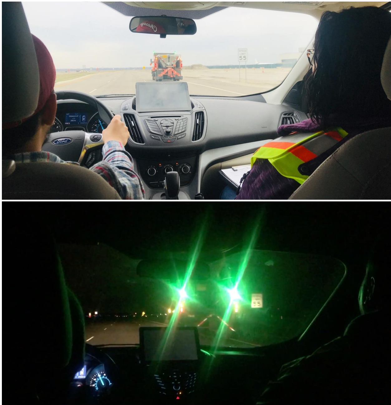
Figure 4-9 Conspicuity, appropriate driving action and glare rating tests in the dynamic experiment
