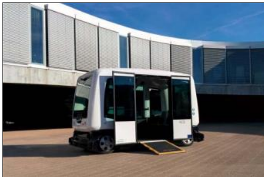
Figure 2 – EasyMile EZ10 with ramp for passengers with reduced mobility (Source: 18)
