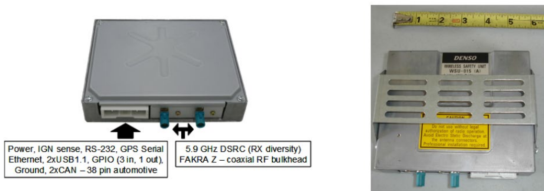
Figure 24. DENSO WSU1.5 with automotive-grade and style connectors
