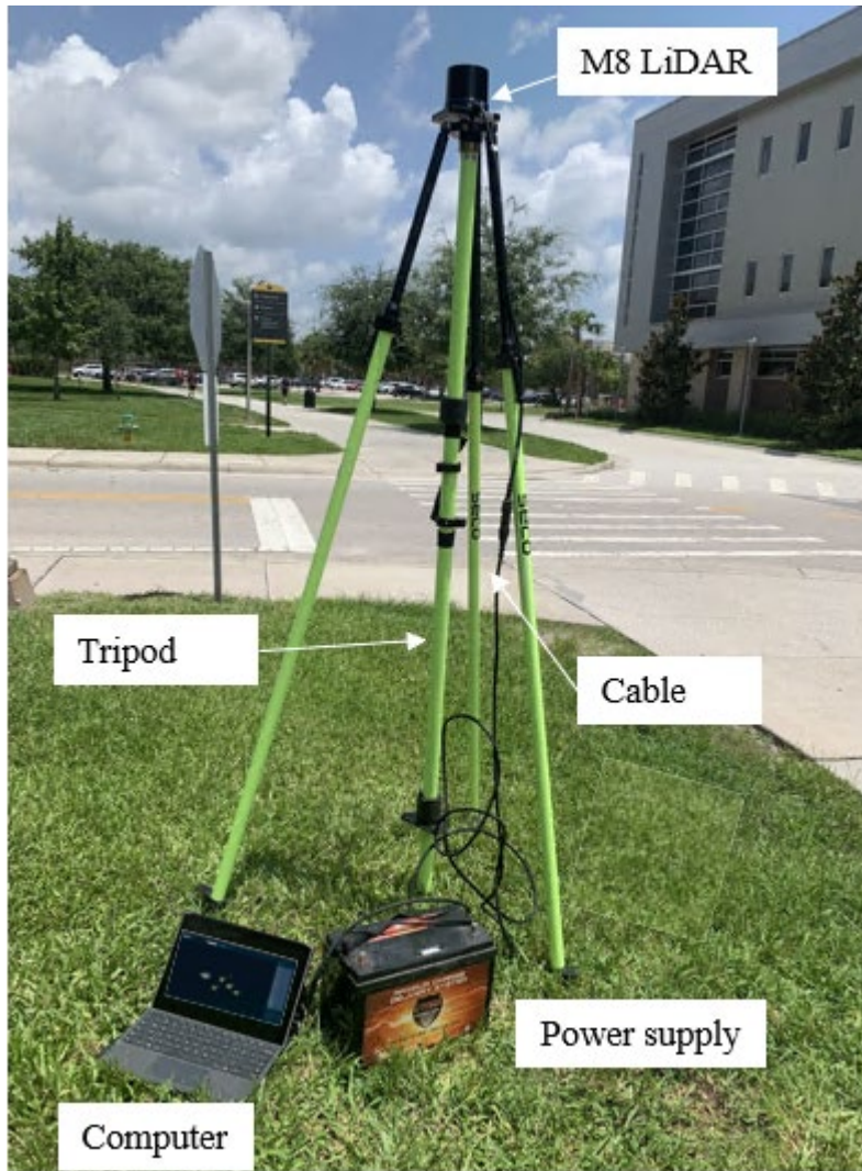
Figure 76. Setup for the M8 LiDAR
