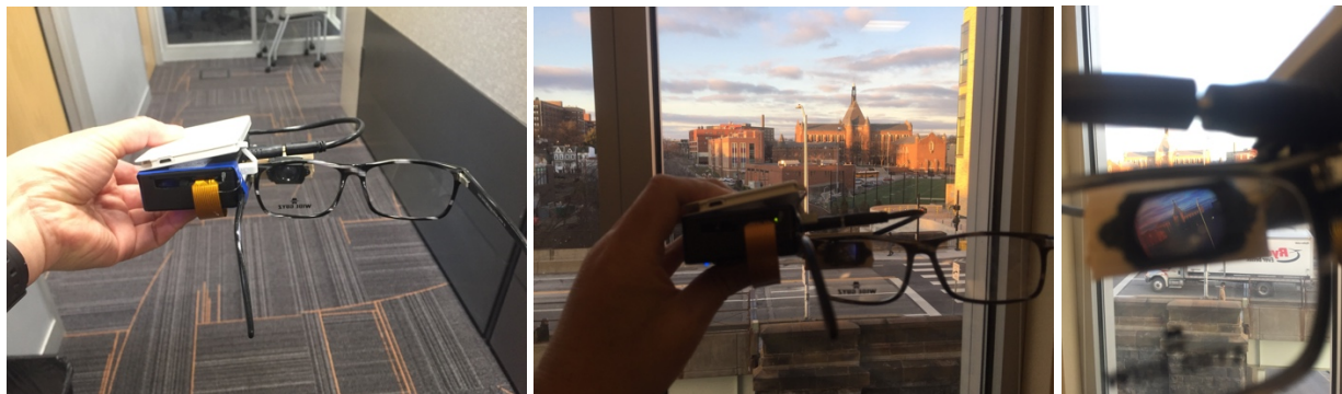
Figure 1. Prototype One: Micro Video HUD (left), test scene of the building in distance (middle) and the HUD view (right)
