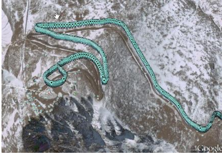
Figure 18. Google Earth Map of Piloted Ascent of Pikes Peak (Datum Shift Present)
