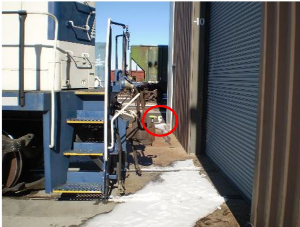
Figure 23. A Mock-up of an EOT Case Constructed to Mount the Antennas
