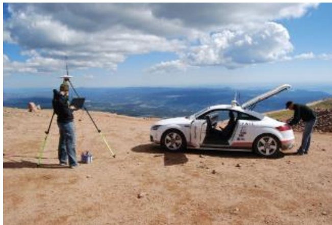
Figure 17. Conventional RTK System Used by the Stanford University Team
