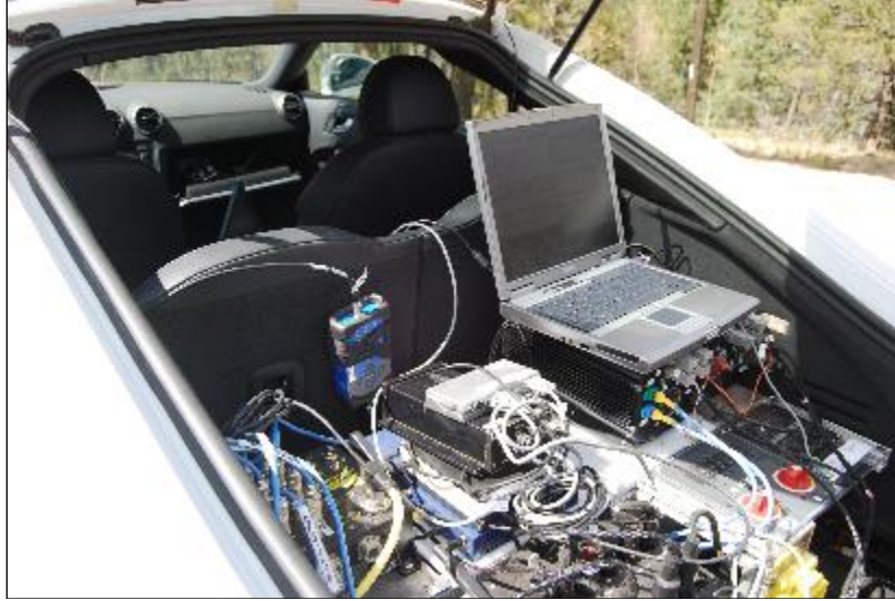
Figure 14. The TTC Laptop and Raven Beacon Receiver Installed on Audi TT
