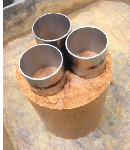
(a) pushing tubes into the soil sample
