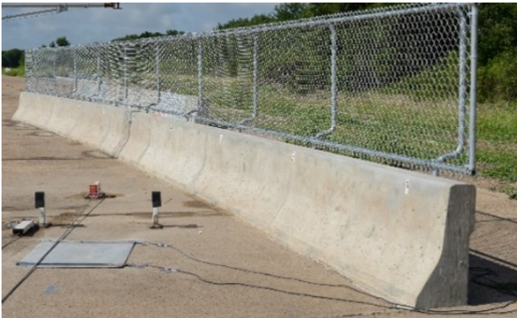
Figure 7. Tested Retrofitted Design on the Test Site.
