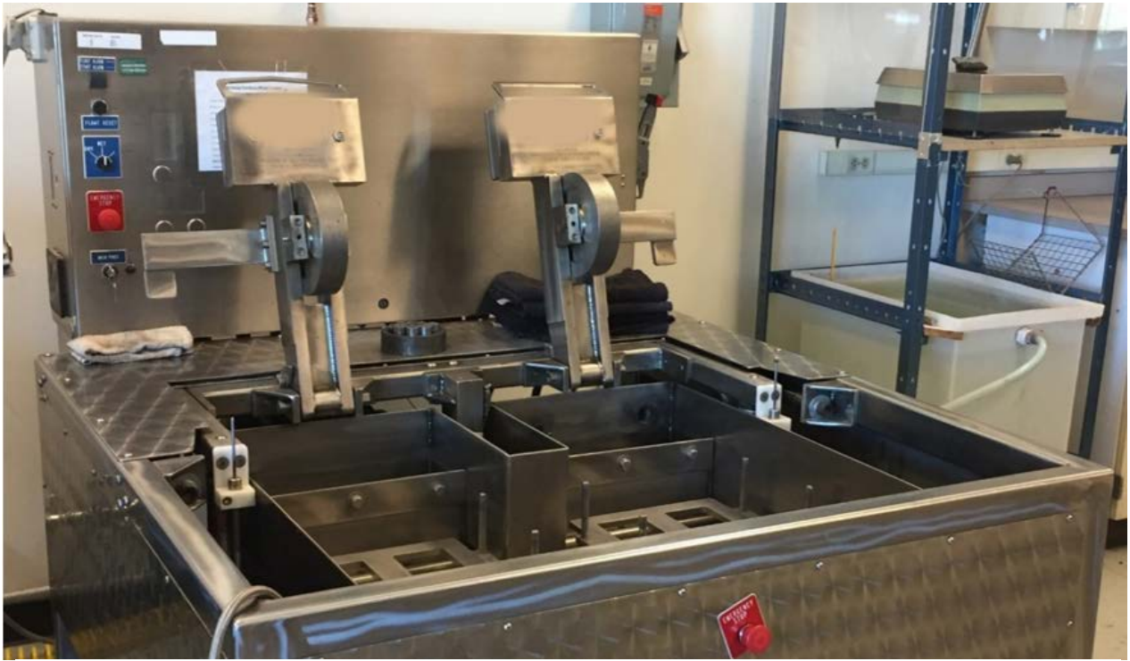
Figure 5. One make and model of a Hamburg wheel-track testing device.
