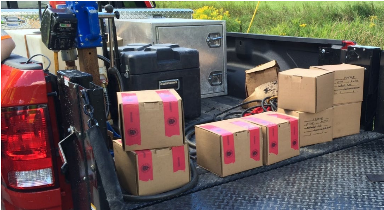
Figure 9. Example of sample security with tamper-proof tape on cardboard sample boxes.
