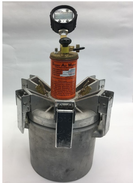
Figure 2. One make and model of Super Air Meter.
