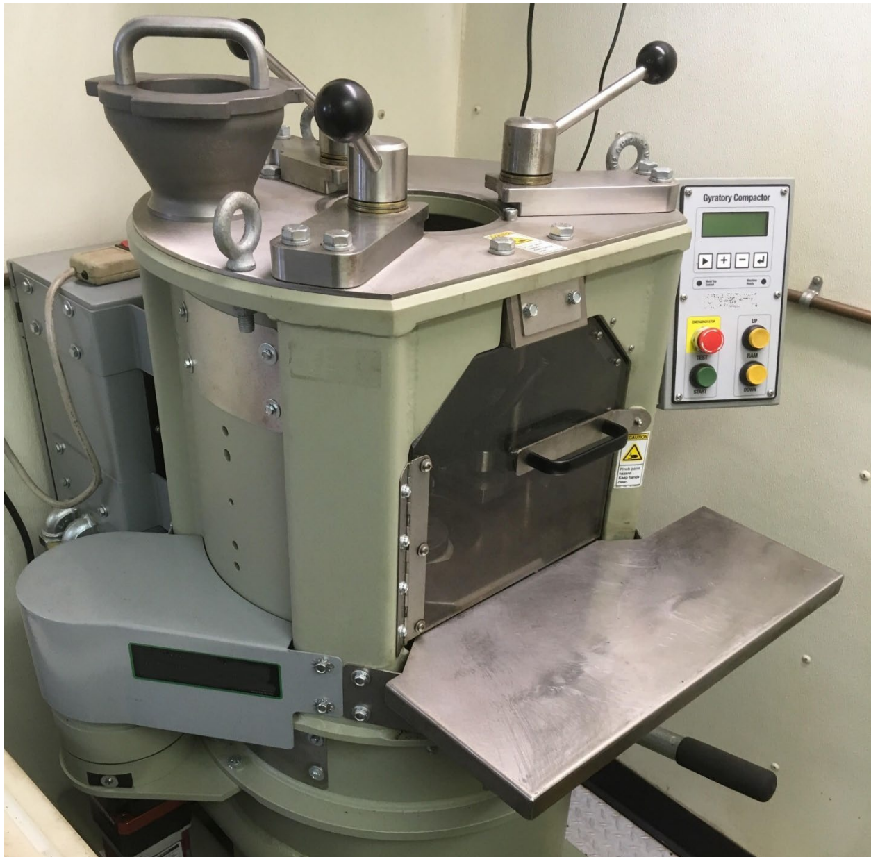
Figure 4. One make and model of a Superpave gyratory compactor.
