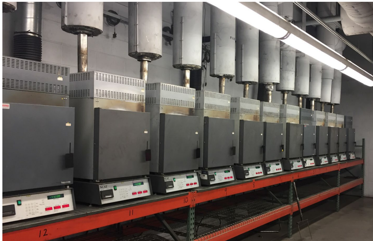
Figure 11. Example ignition furnace setup at an SHA laboratory.
