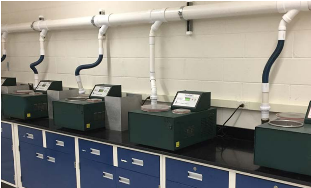
Figure 10. Example setup of rapid material sample drying equipment used by an SHA.
