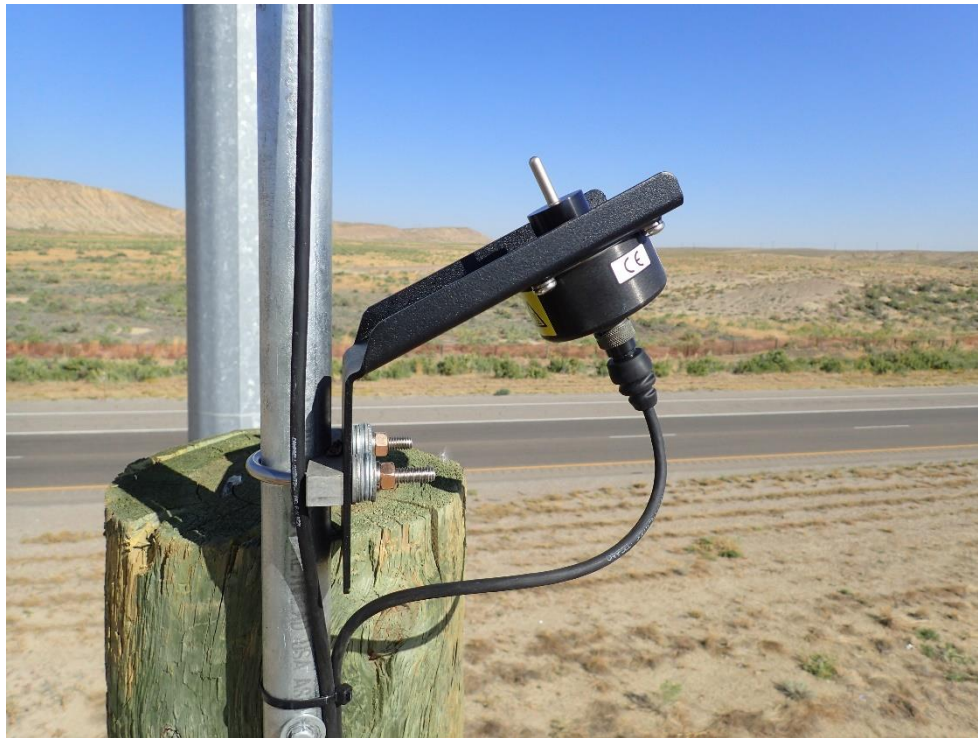
Figure 16. Freezing rain sensor and mounting kit
