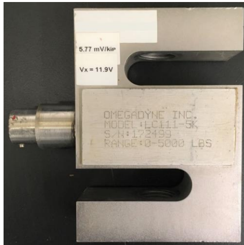
Figure 20. Omega Dyne Model LC111-5k Stainless S-Beam Load Cell
