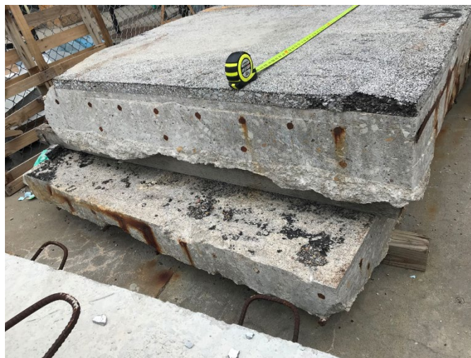
Figure 45. Field Specimen. View from South End showing the nine rebars
