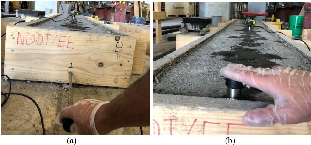
Figure 18. Two longitudinal continuous test setups: (a) UGWL Method application. Transmitter on the end of rebar and receivers along the middle line on the asphalt surface ( Results in Figure 19 ). (b) Indirect UPV Application. Transmitter on the asphalt surface 2 inches from the edge and receivers along the middle line on the asphalt surface ( Results in Figures 20-21 ).
