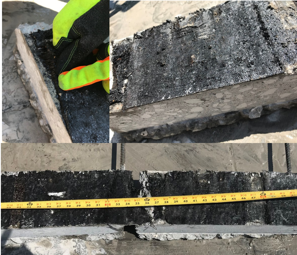
Figure 30. Segment B2: Status of Membrane After Testing
