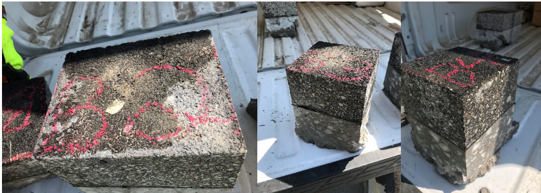
Figure 12. Density test was conducted on the sliced segments of Specimen B
