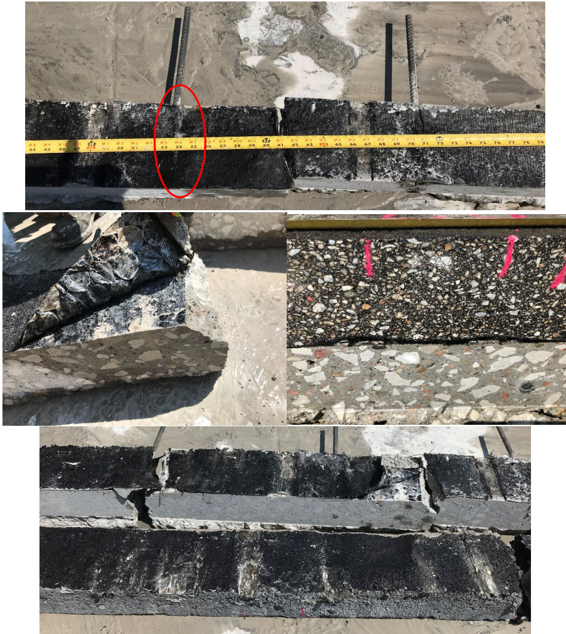
Figure 32. Segment B3: Status of Membrane After Testing
