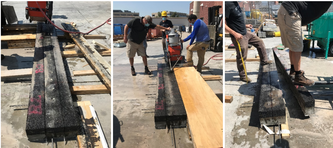
Figure 26. Dissecting Specimen B to evaluate the asphalt-membrane-concrete interface
