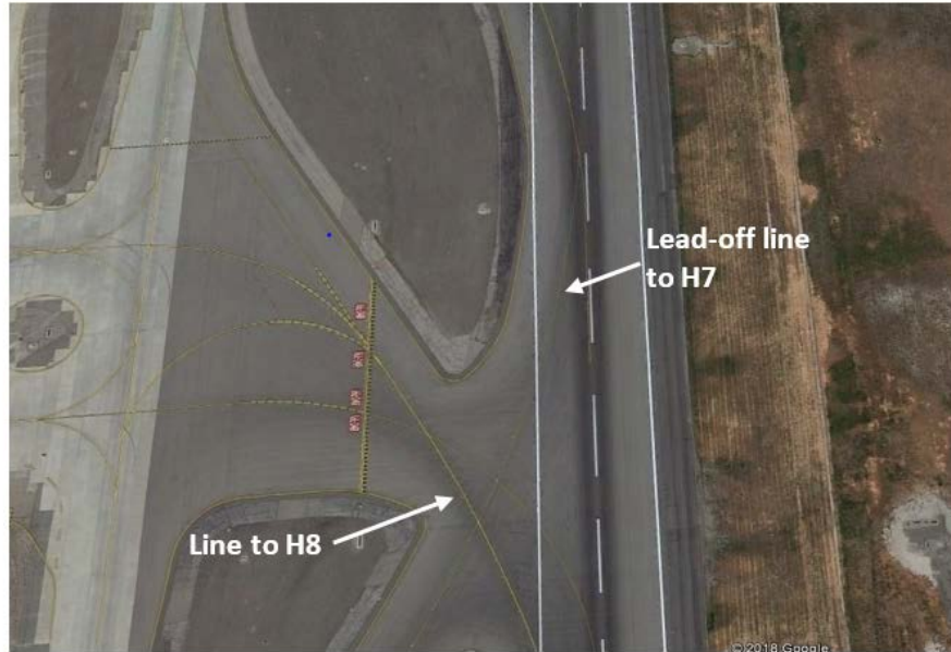
Figure 5. Layout of intersection 3 and lead-on/lead-off lines.
