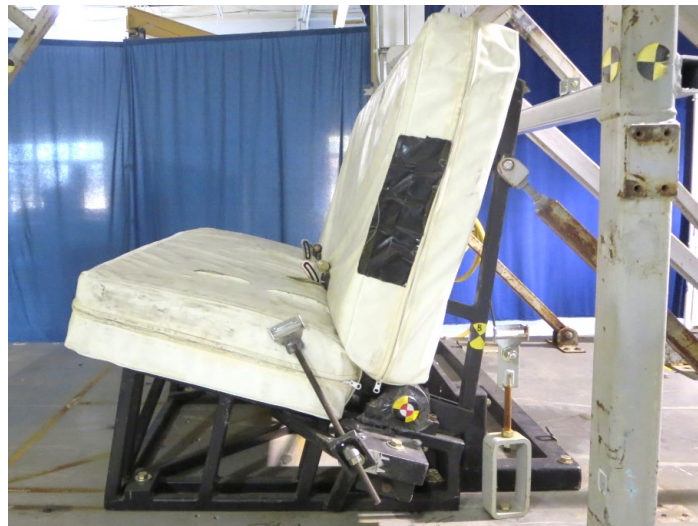
Figure 1: FMVSS No. 213 Standard Seat Assembly-Current Test Buck
