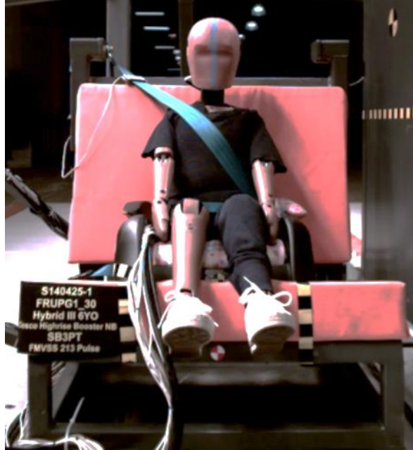
Figure 9: Seat Back Height With Low Back Booster
