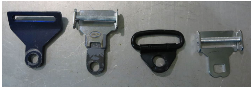
Figure 3: V2 Anchorage Hardware
