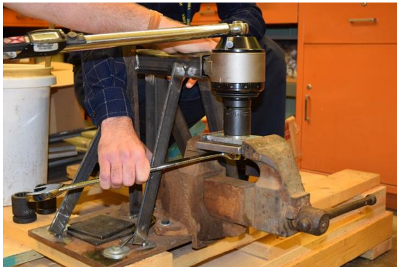
Figure 15. Fixture Used for Bolt Installation on Long-Term Corrosion Test Specimens
