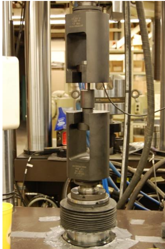
Figure 3. Photograph Showing Bolt Testing Fixture
