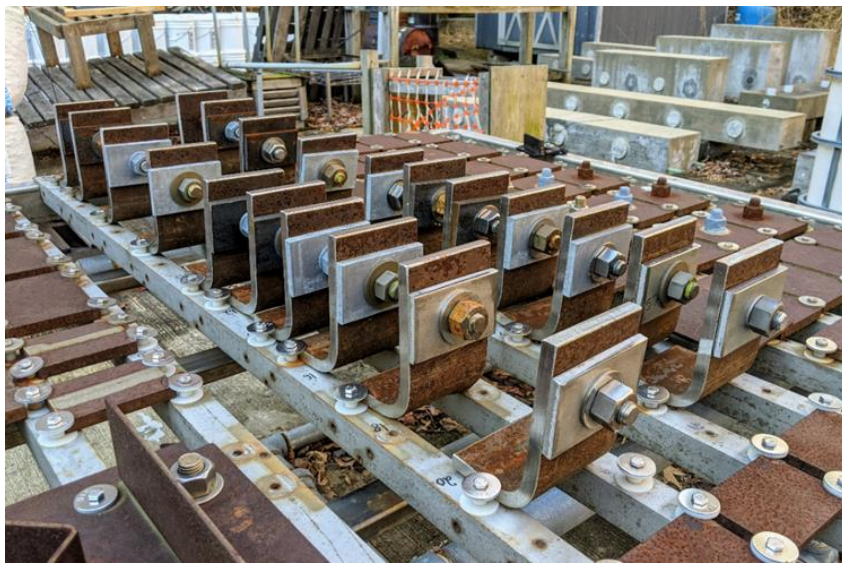
Figure 45. Photograph of Corrosion-Resistant Fastener Long-Term Corrosion Test Specimens
