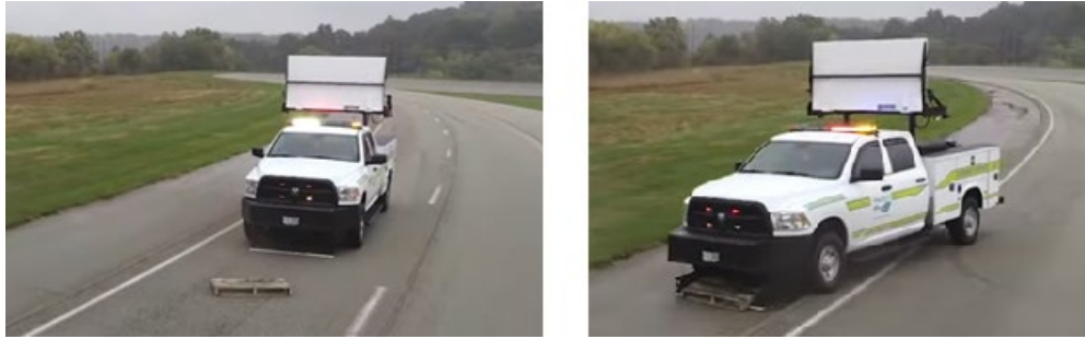
Figure 29. JAWS mounted truck removes debris to shoulder
