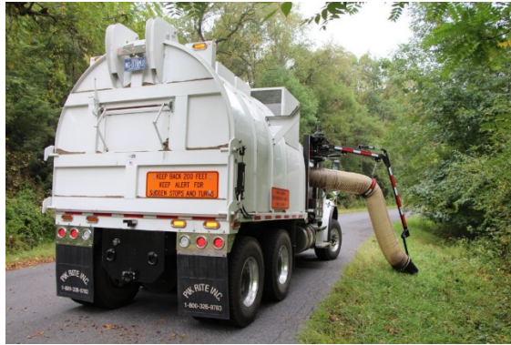
Figure 27. Pik Rite Truck Mounted Debris Collector
