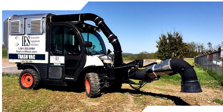
Figure 25. Trash Vac by Neptune Wash Solution
