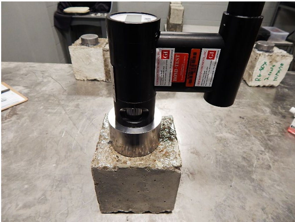
Figure 54: Example of Pull-off Testing
