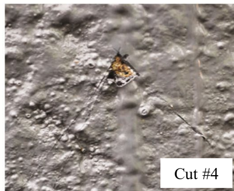
Figure 44: Testing: Five V-notch knife cuts were made with a box cutter on product 4
