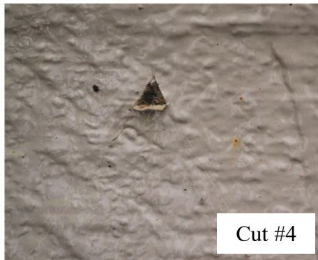
Figure 42: Testing: Five V-notch knife cuts were made with a box cutter on product 2
