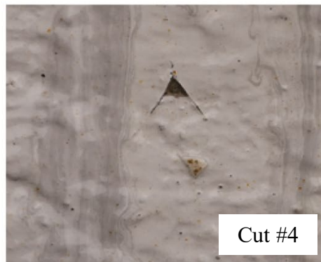
Figure 41: Testing: Five V-notch knife cuts were made with a box cutter on product 1
