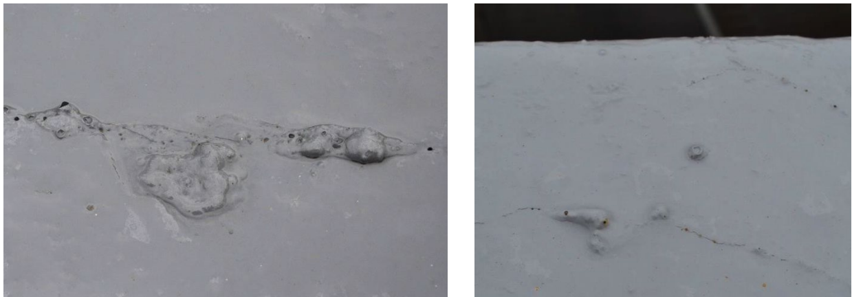
Figure 53: Bubbled polyaspartic product observed after one winter
