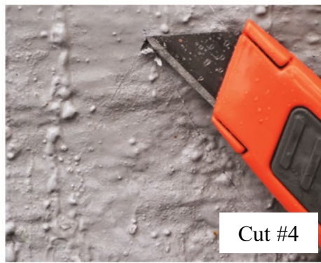
Figure 43: Testing: Five V-notch knife cuts were made with a box cutter on product 3
