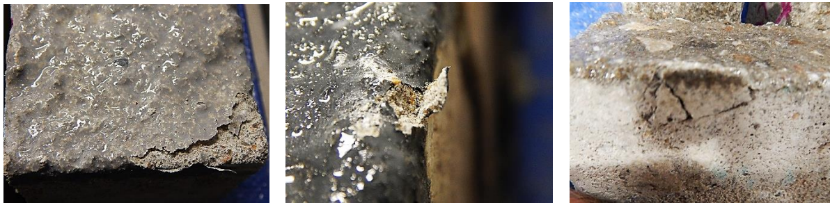
Figure 93: Freeze-thaw distress features: edge deterioration and scaling retained by coating, a) DYNA-PUR7416, b) DYNA-PUR7416 NT6 and c) Mirabel Fast products
