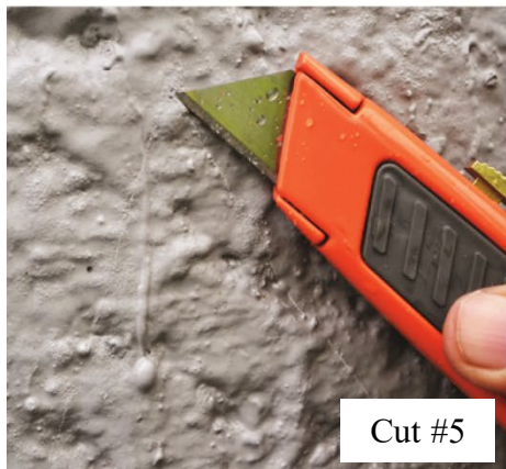
Figure 43: Testing: Five V-notch knife cuts were made with a box cutter on product 3
