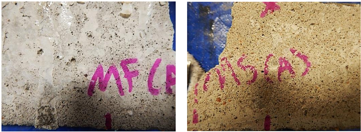
Figure 92: Freeze-thaw distress features: concrete surface deterioration and mortar flaking a) Mirabel Fast and b) Mirabel Slow products
