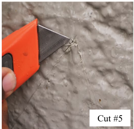
Figure 42: Testing: Five V-notch knife cuts were made with a box cutter on product 2
