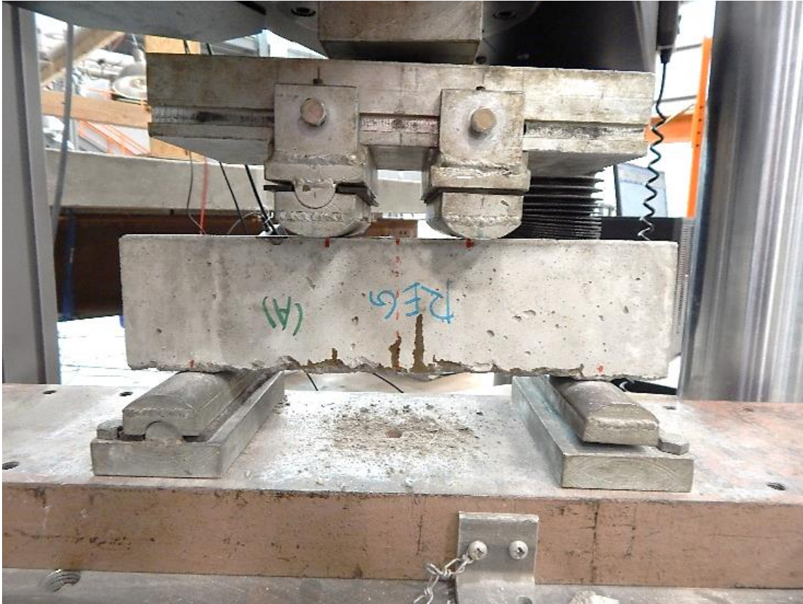
Figure 55: Flexural test setup
