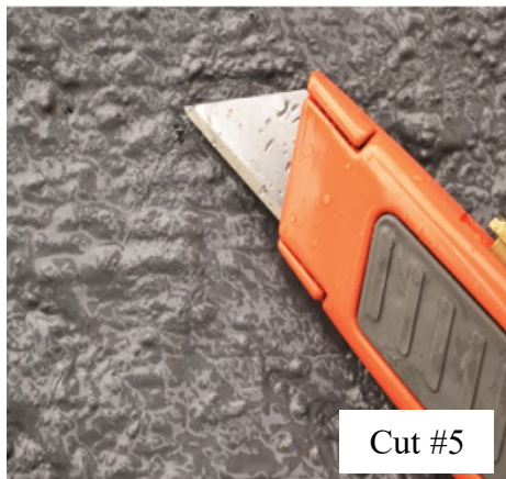
Figure 44: Testing: Five V-notch knife cuts were made with a box cutter on product 4
