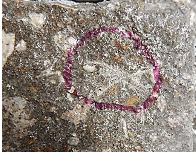
Figure 98: Example of V-notched test result: Rust-Oleum RG-80X product
