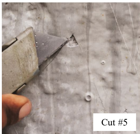
Figure 41: Testing: Five V-notch knife cuts were made with a box cutter on product 1
