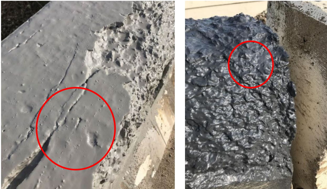
Figure 39: Air bubbles found in product 1 and product 4 after Application No. 1 on SR142
