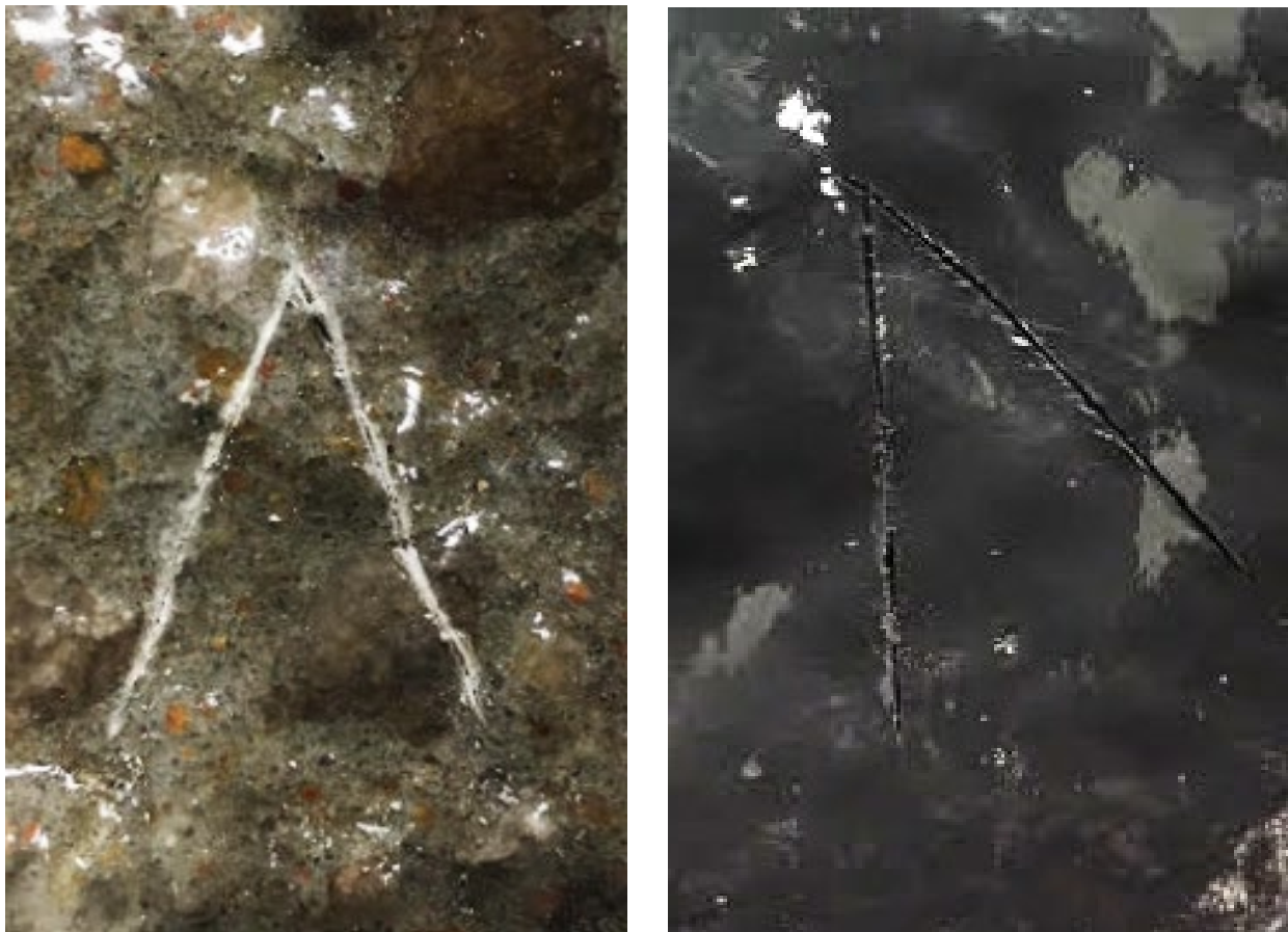
Figure 40: Example V-notch cuts on polyaspartic samples in the laboratory
