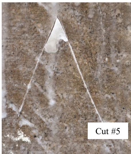
Figure 45: Testing: Five V-notch knife cuts were made with a box cutter on product 5
