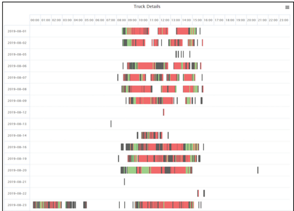
Figure 6.8 Daily utilization dashboard for a single maintenance vehicle.
