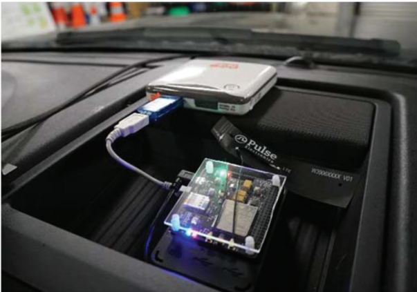
Figure 7.1 Raspberry Pi device for receiving CAN messages from Wi-Fi.
