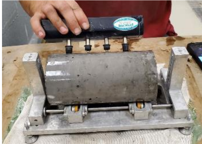
Fig 3.20 Surface resistivity specimen being tested.
