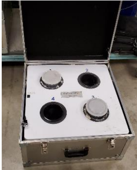
Fig 3.7 SAT specimens placed inside the semi-adiabatic calorimeter chamber.
