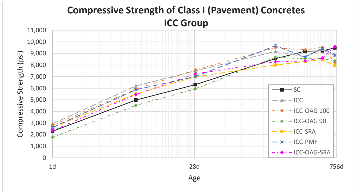
Fig 3.24 Compressive Strength of Class I (Pavement) Concretes, ICC group.
