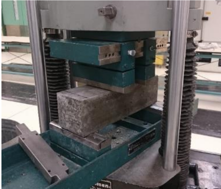
Fig 3.12 Flexural strength specimen being tested.
