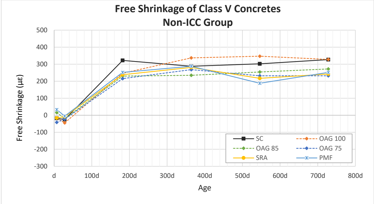
Fig 3.63 Free shrinkage of Class V Concretes, non-ICC group.
