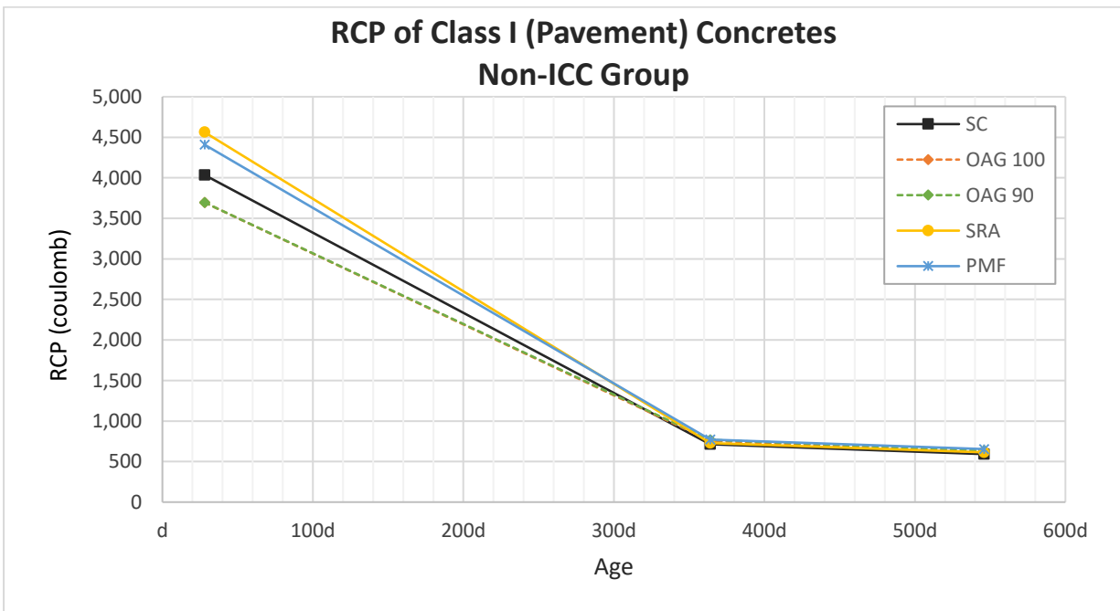
Fig 3.68 RCP of Class I (Pavement) Concretes, non-ICC group.
