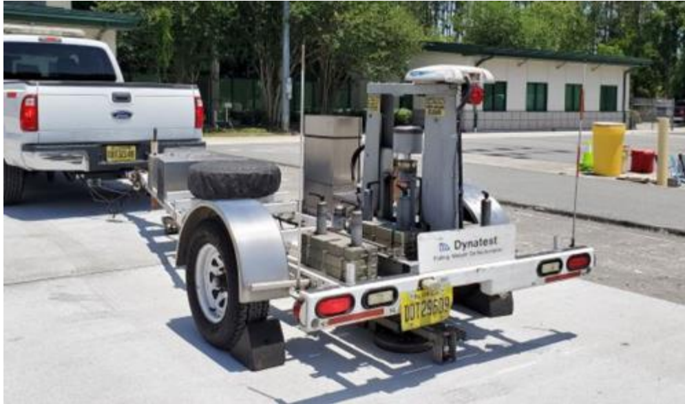
Fig 5.9 FWD testing on the slab.
