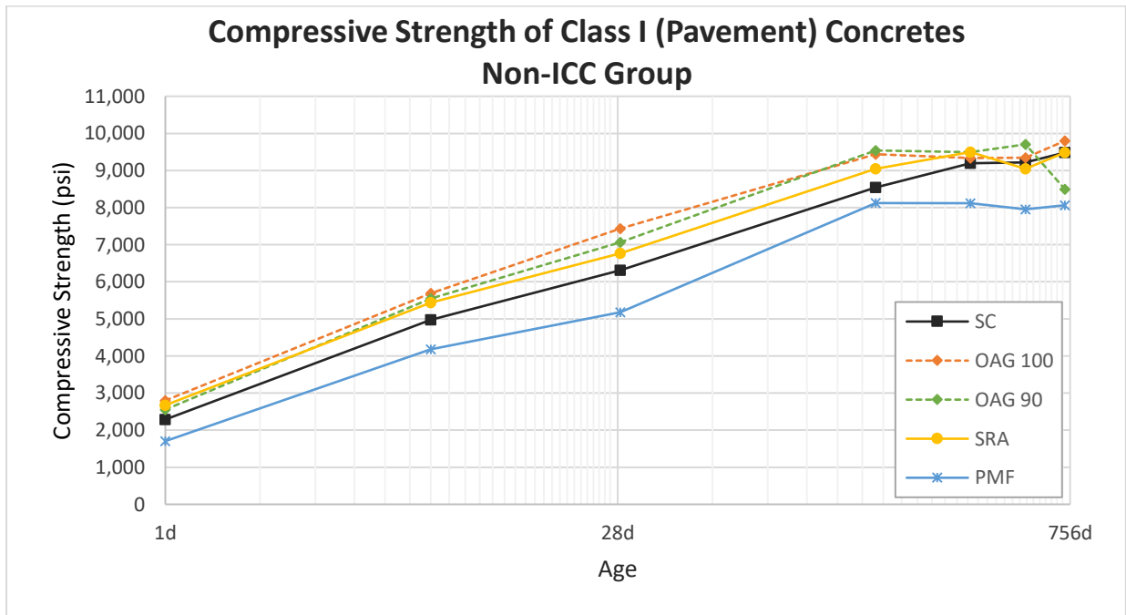
Fig 3.23 Compressive Strength of Class I (Pavement) Concretes, non-ICC group.
