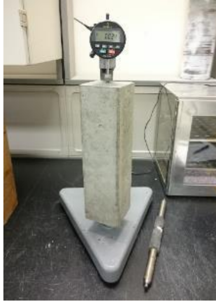
Fig 3.15 Free-shrinkage specimen being tested.
