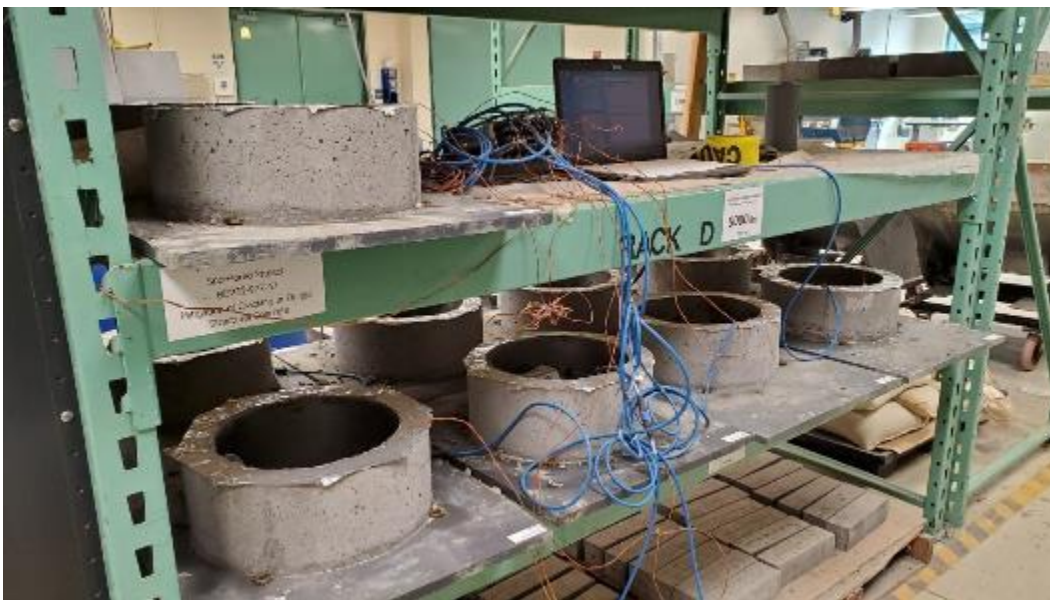
Fig 3.18 RSR specimens being tested.
