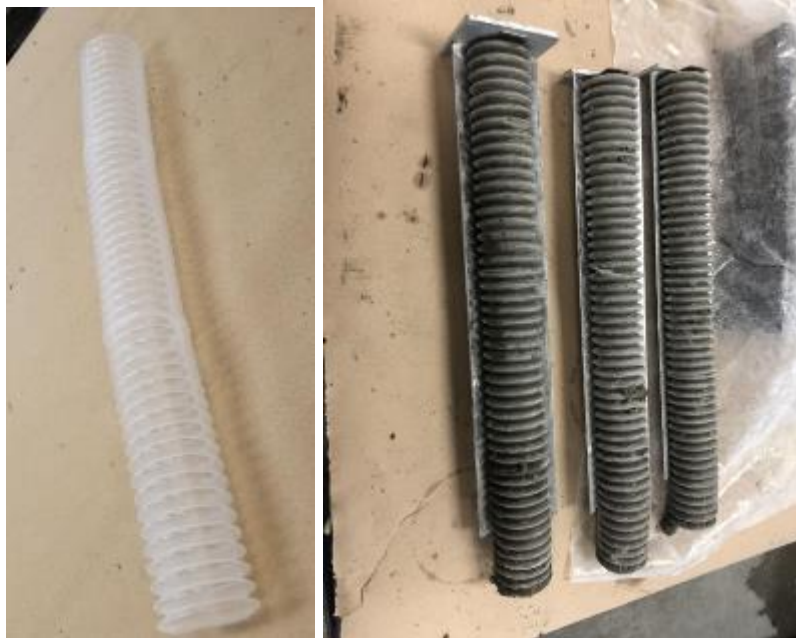
Fig 3.16 Three-inch diameter corrugated tube (left) and autogenous shrinkage specimens (right).
