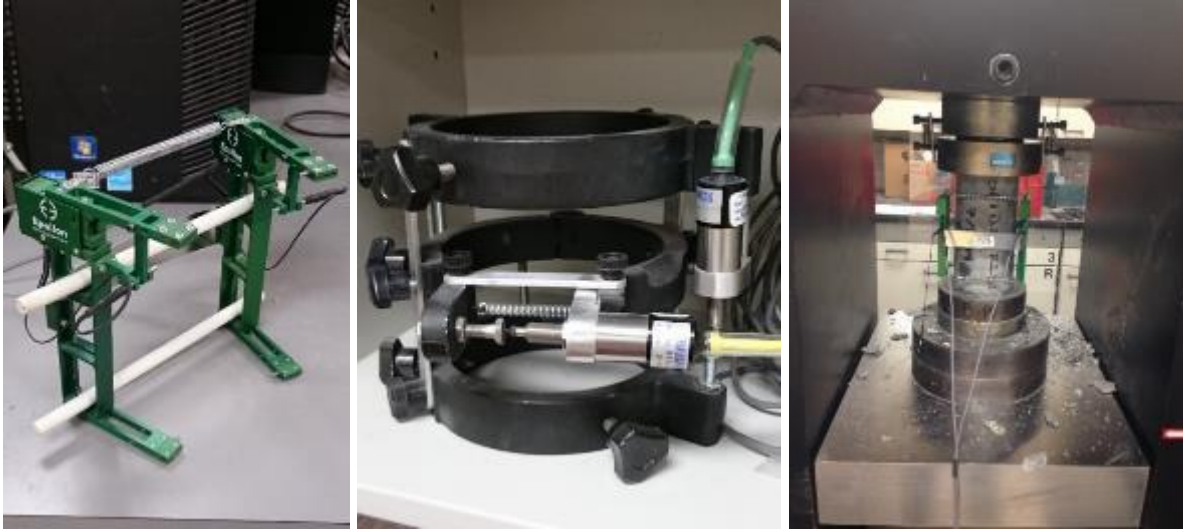
Fig 3.13 Compressometer and extensometer apparatus for MOE test (left), traditional MOE apparatus (middle), and the MOE specimen being tested (right).
