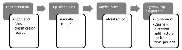
Mode choice considers premium versus non-premium modes; premium includes heavy rail and express bus. The four-step model does include a feedback loop based upon a convergence criterion. Congested travel times are fed back using an MSA approach.
