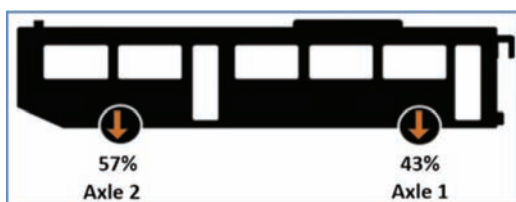
Figure 4.2 Axle load distribution on two axles.
