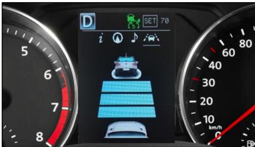
Figure 5. Close-up of ACC interface
