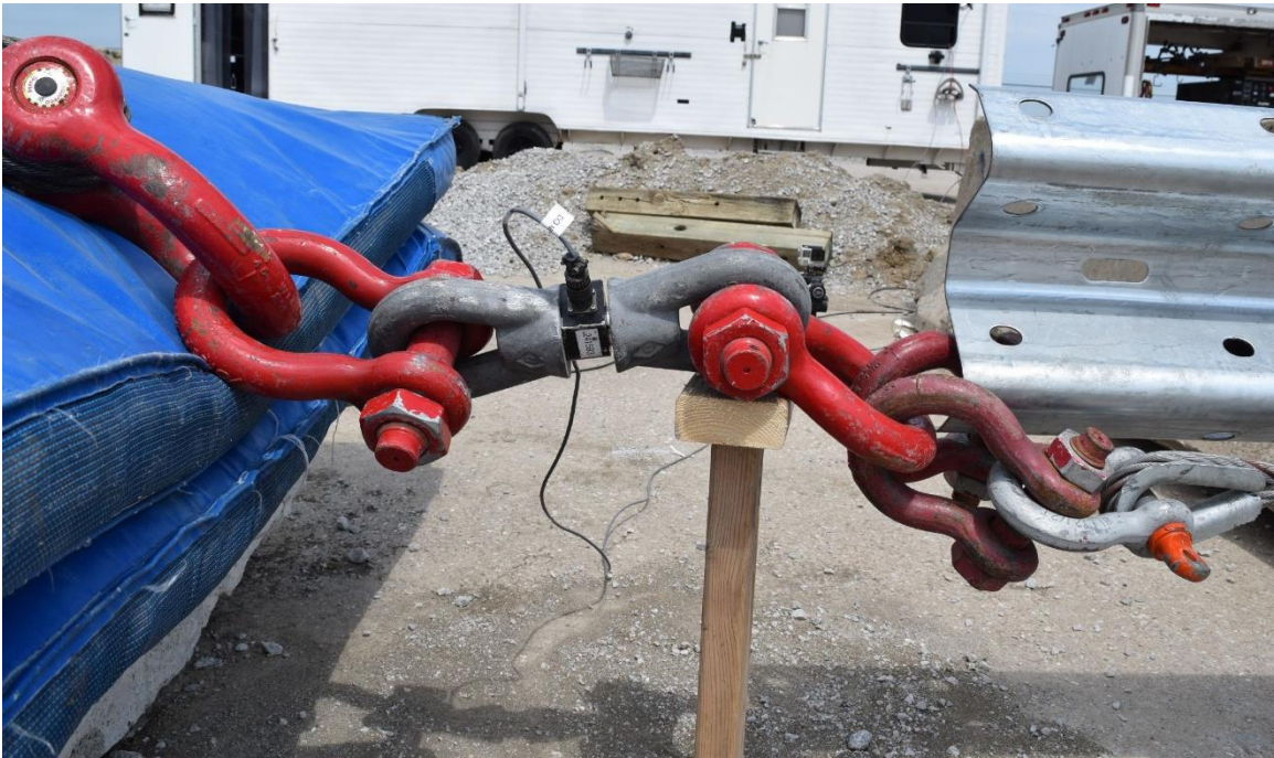
Figure 65. Tensile Load Cell Setup, Test No. SPDA-4
