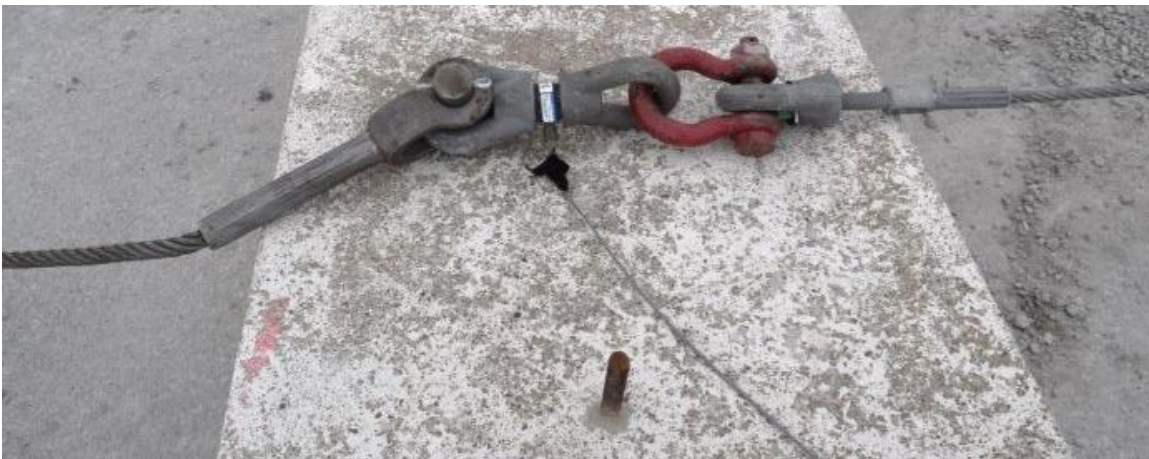
Figure 63. Tensile Load Cell Setup, Test No. SPDA-2
