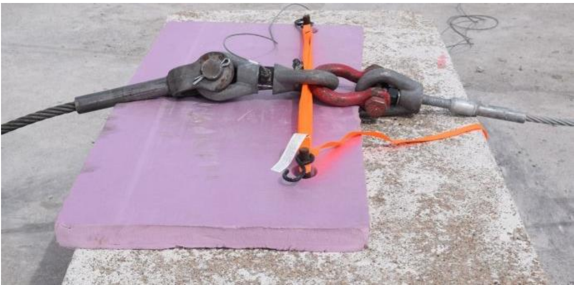
Figure 62. Tensile Load Cell Setup, Test No. SPDA-1
