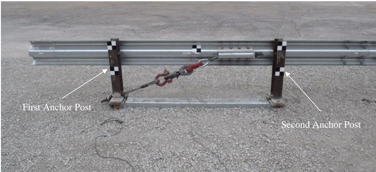
Figure 136. Test Setup, Test No. SPDA-3
