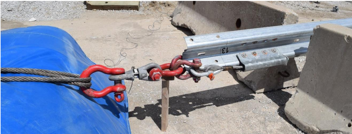
Figure 66. Tensile Load Cell Setup, Test No. SPDA-5
