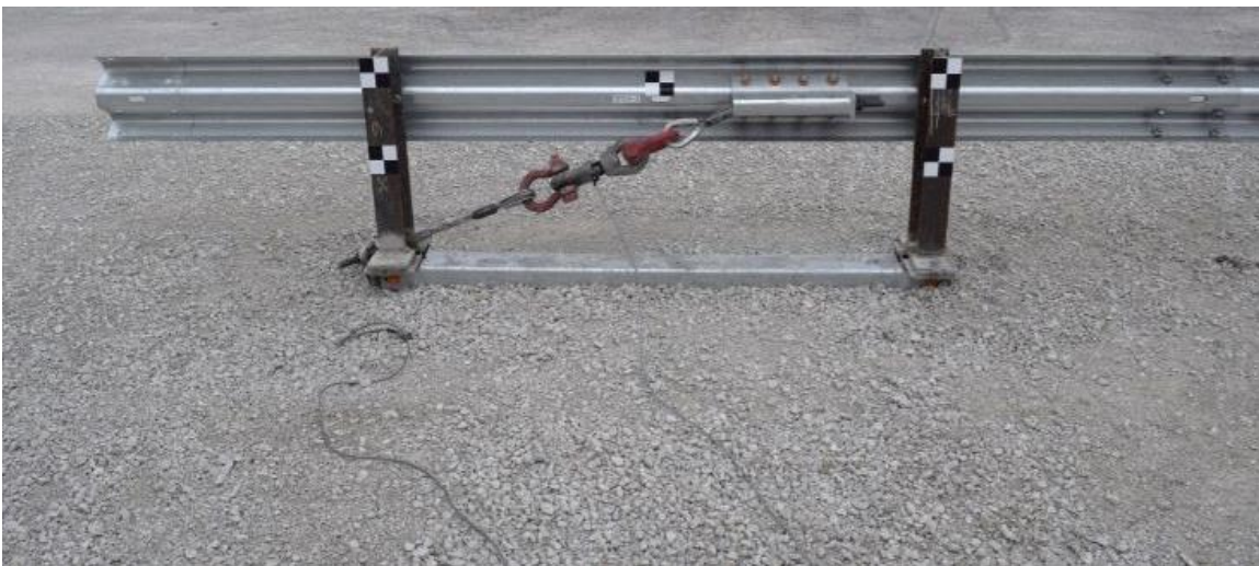
Figure 64. Tensile Load Cell Setup, Test No. SPDA-3
