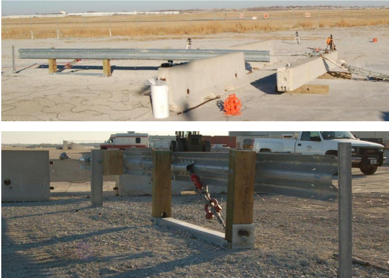
Figure 10. Test Setup: Test Nos. DSAP-1 and DSAP-2 [4]
