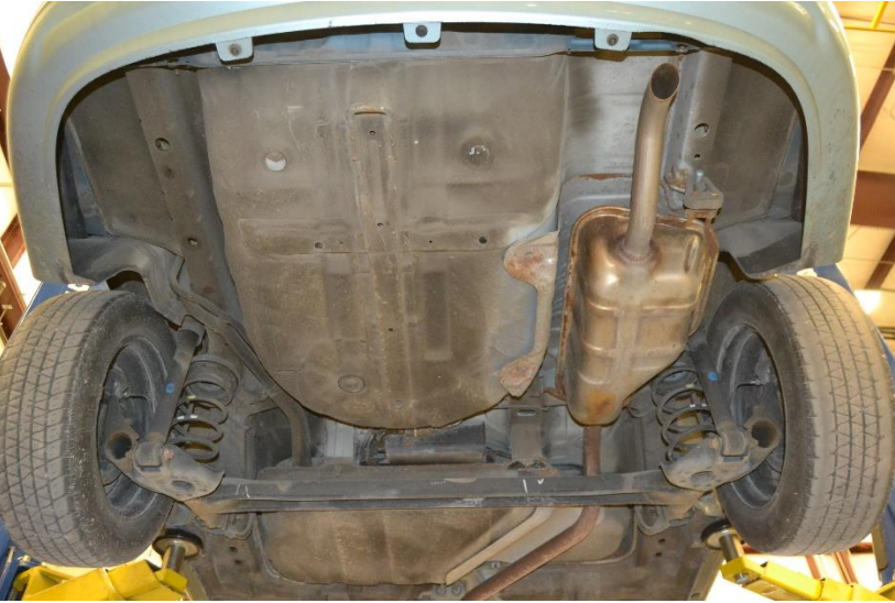
Figure 62. Vehicle Undercarriage Damage, Test No. MGSC-7
