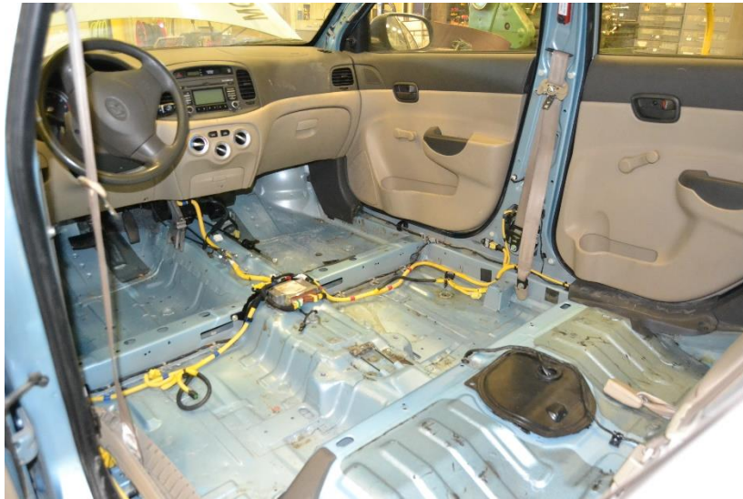
Figure 61. Occupant Compartment Damage, Test No. MGSC-7
