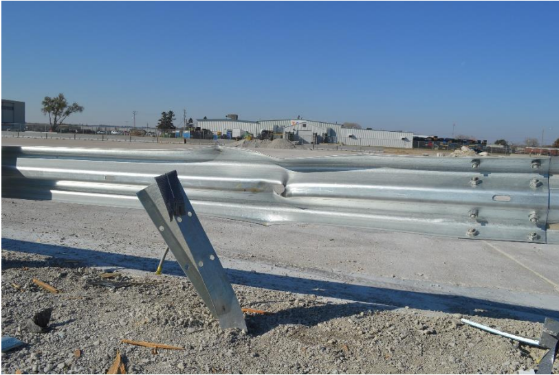
Figure 53. Backside Guardrail Damage, Post Nos. 16 through 18, Test No. MGSC-7
