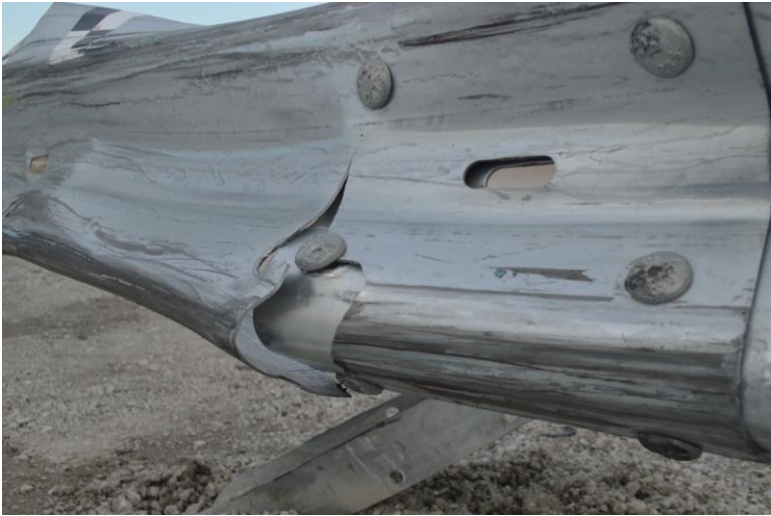
Figure 56. Partial Rail Tearing, Test No. MGSC-7
