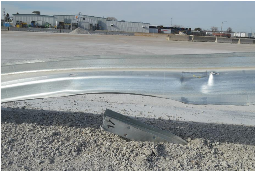
Figure 76. System Damage, Backside Rail at Post Nos. 16 through 19, Test No. MGSC-8
