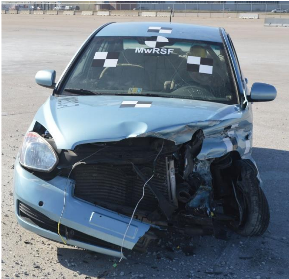
Figure 59. Vehicle Damage, Test No. MGSC-7
