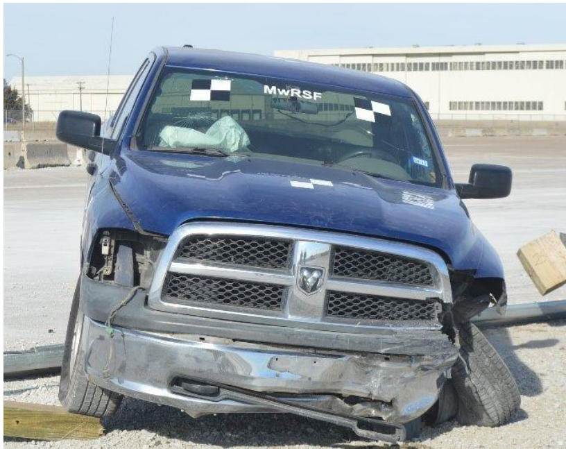
Figure 81. Vehicle Damage, Test No. MGSC-8
