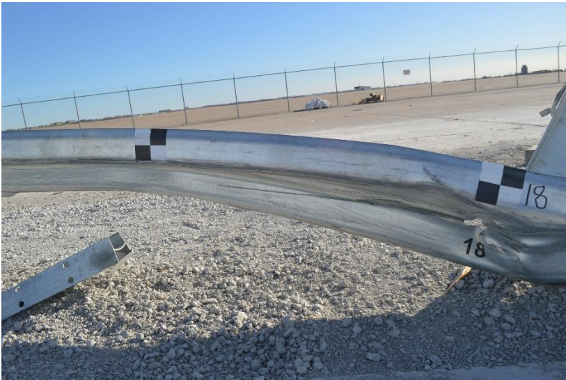
Figure 74. System Damage, Guardrail at Post Nos. 17 through 19, Test No. MGSC-8
