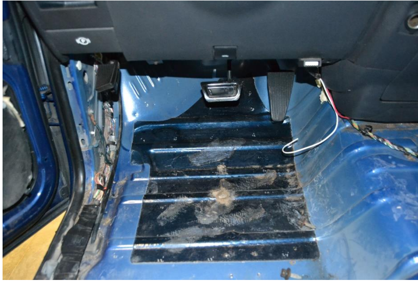
Figure 84. Occupant Compartment Damage, Test No. MGSC-8
