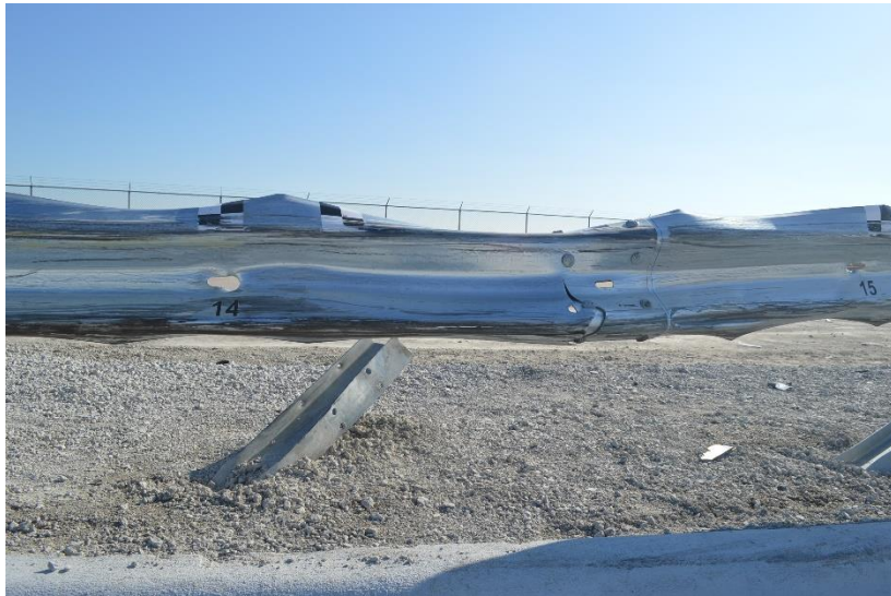
Figure 50. Guardrail Damage, Post Nos. 13 through 15, Test No. MGSC-7
