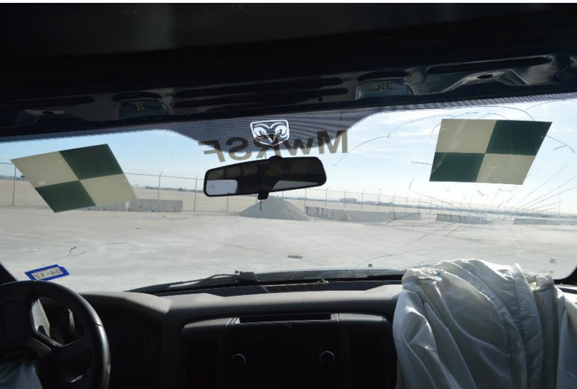
Figure 83. Vehicle Windshield Damage, Test No. MGSC-8
