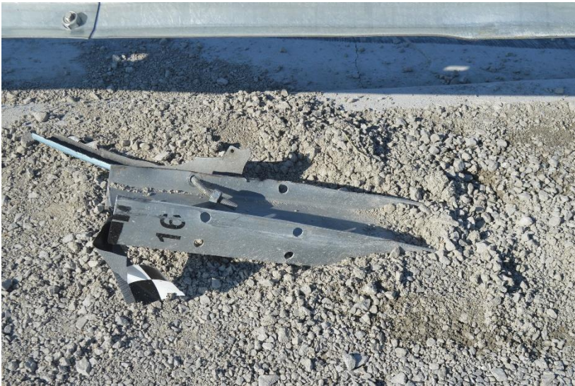
Figure 55. Post Nos. 16 and 17 Damage, Test No. MGSC-7
