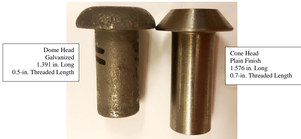
Figure 1. Illustration of Differences between Sleeve Nut Concepts
