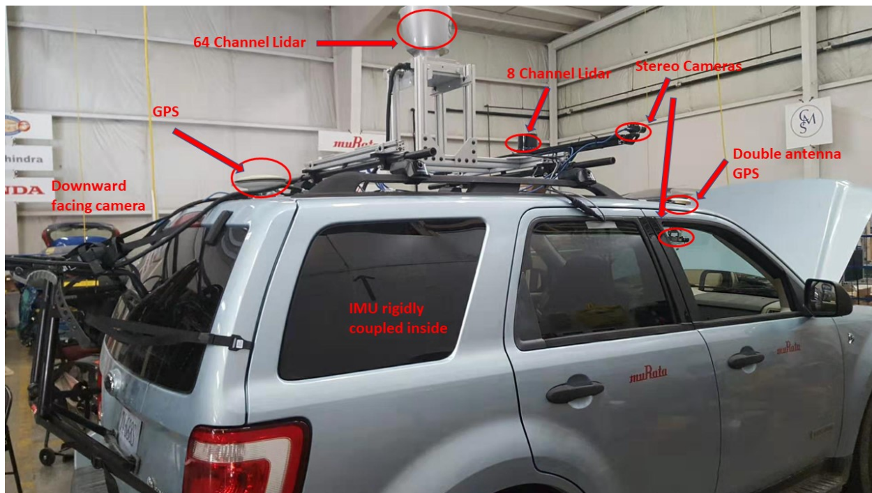
Figure 15. Equipment installation picture of the test vehicle.
