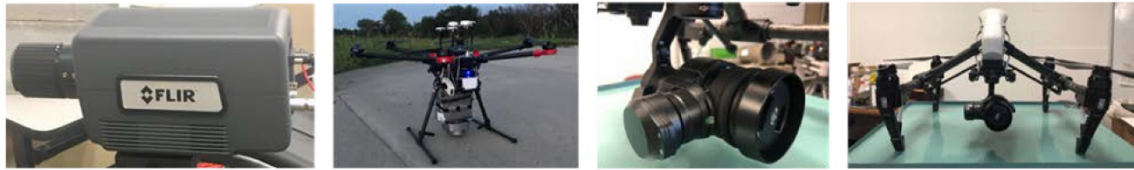
Figure 4. Equipment used for field data acquisition of bridge decks (Left to right: FLIR A8300 camera, DJI M600 drone, DJI X5 camera, and DJI Inspire 1 drone)
