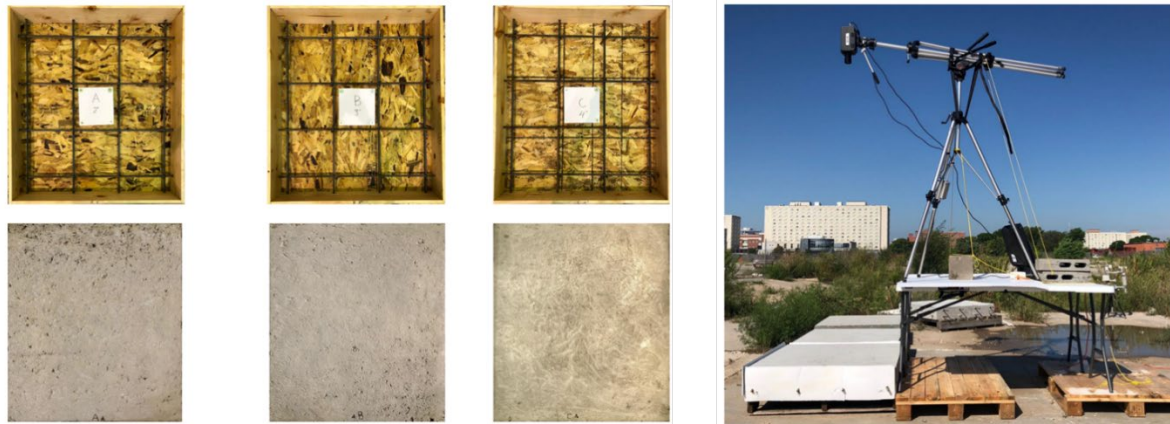
Figure 9. Experimental Specimens and IRT image recording settings.
