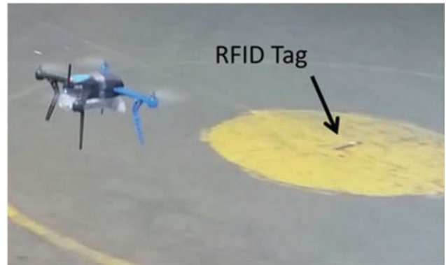
Figure 6.18 UAS mounted with RFID reader to identify RFID tag.
