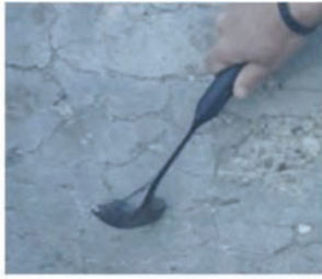
(a) Hammer sounding can be used on concrete and timber (Triplett & Jordan, n.d.).
