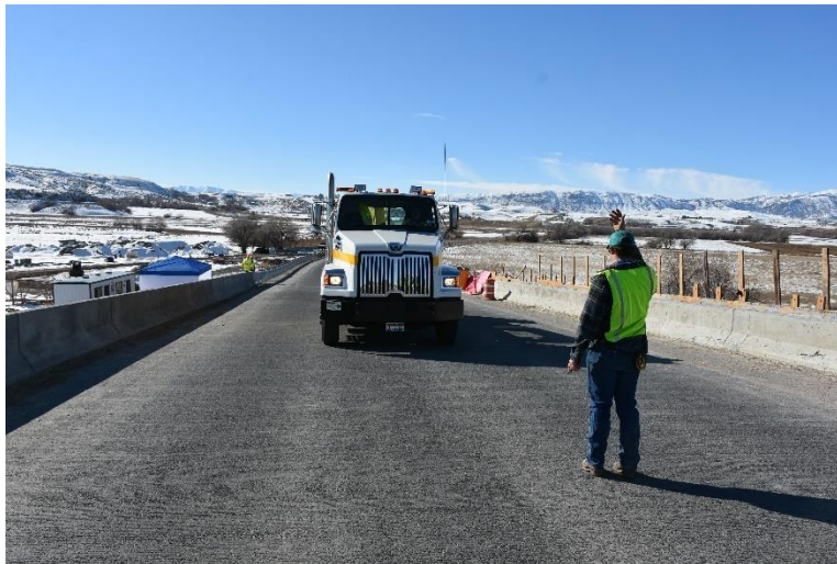
Figure 41. UBIT static loading.
