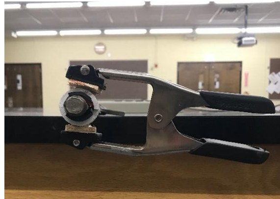
Figure 10. Rebar clamping technique.
