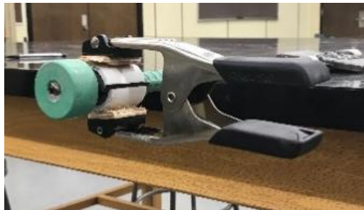
Figure 2. Rebar clamping procedure.
