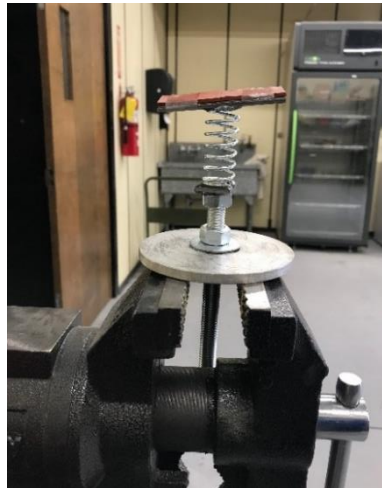
Figure 18. Spring clamping device.
