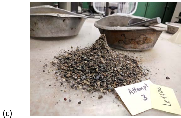
Figure 14 Various stages of the cone, (a) Stage 1 – aggregate is too wet, (b) Stage 2 – SSD condition, (c) Stage 3 – Drier than SSD condition
