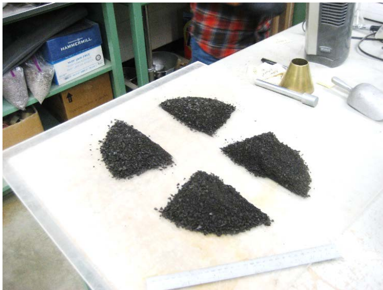
Figure 15 Quartering of SSD aggregate sample
