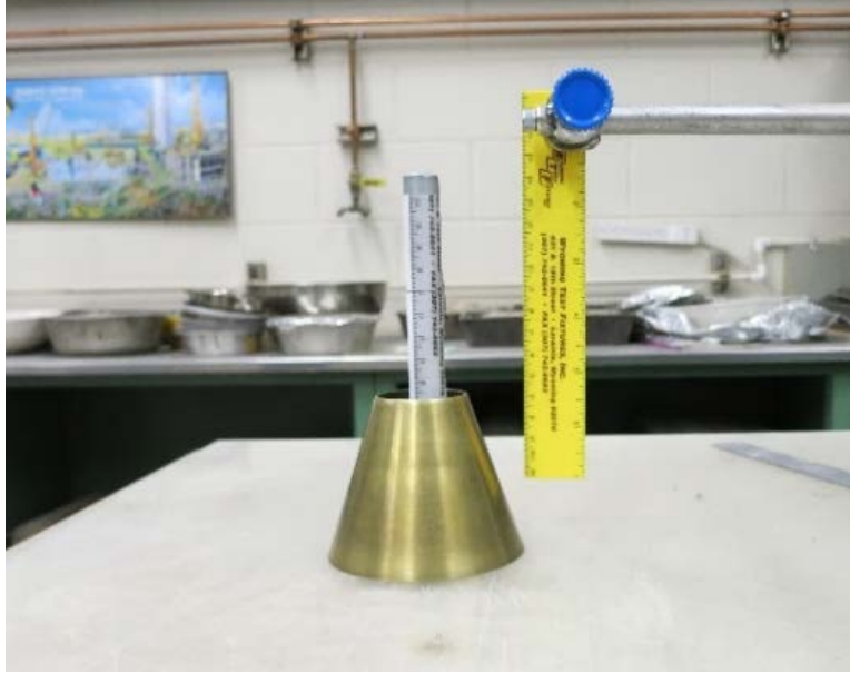
Figure 19 Test for tamper drop height
