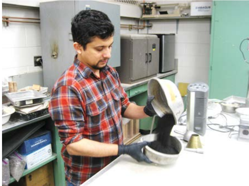
Figure 12 Drying of sample using pans
