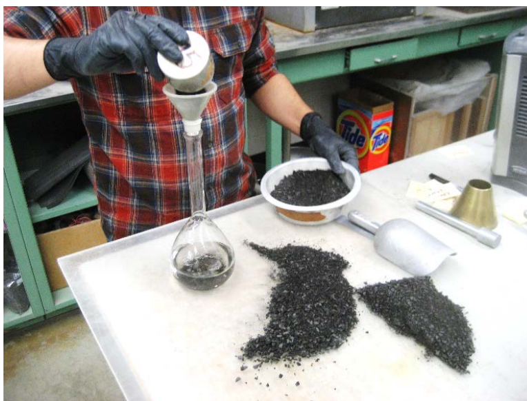
Figure 16 Pouring of SSD samples for de-airing
