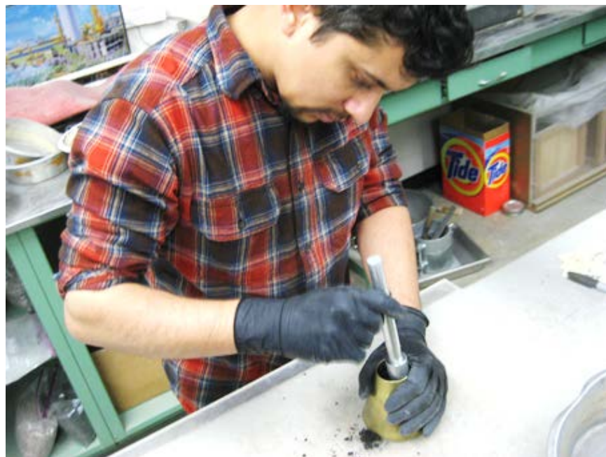
Figure 13 Tamping aggregate into cone
