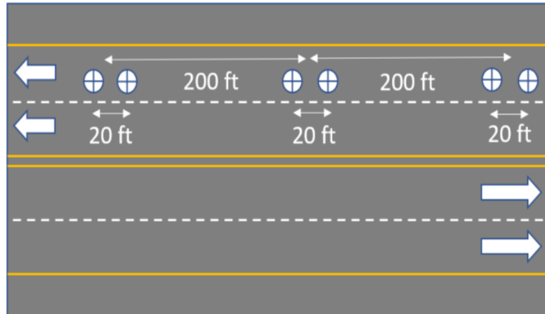
Figure 31. Schematic for Locations of DFT and Sand Patch Measurements
