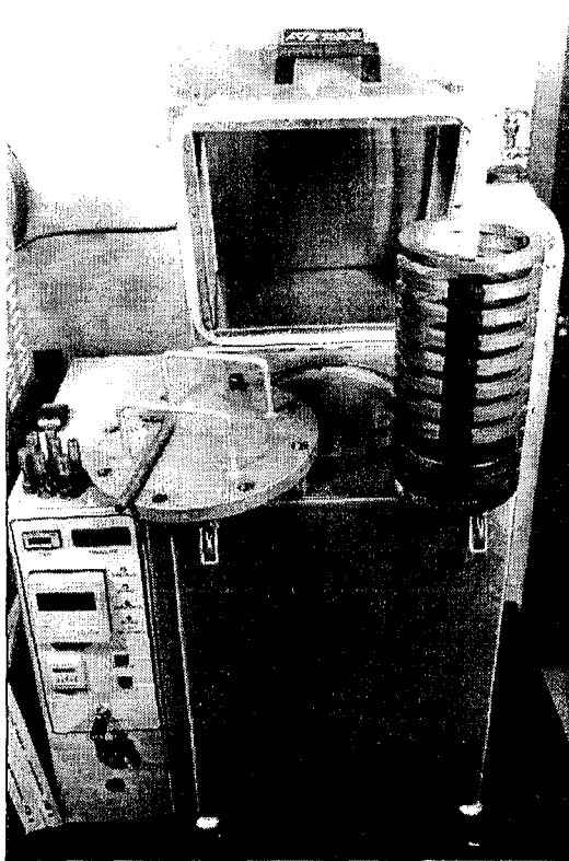
Pressure Vessel Built into Oven
